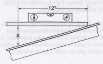
the distance from the roof surface to the underside of board to calculate exact roof pitch. EXAMPLE: If "X" = 3-3/4", your roof pitch is 3-3/4"-in-12".
