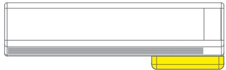
The Gobi II pump can be mounted on the right or left side of an evaporator unit.
