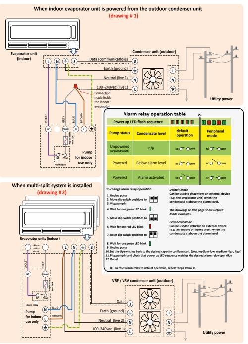
Below are examples of how REFCO pumps can be installed. For reference only.
