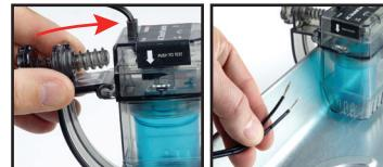
3. Tighten the thumbscrew to hold the switch in place and route the wires neatly to the air-handler or furnace.
