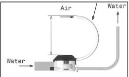
Black cap must be fitted on the unused outlet.
