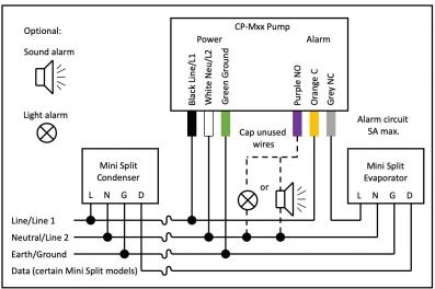
Installation of the Pump Module
