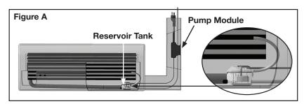
The power must be connected to a different source than air unit. Disconnect power before installation. Only use the supplied cables.
