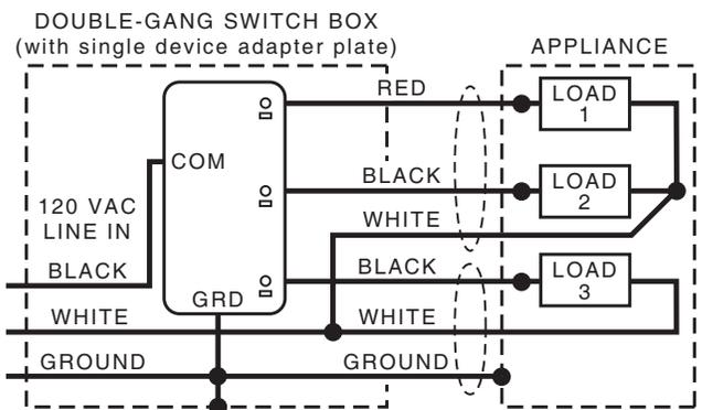
**4B. When using a 2-Rocker Switch to turn a range hood ON & OFF from another location with 120 VAC POWER CABLE ENTERING SWITCH BOX:**
