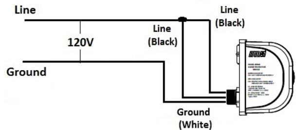
**Installation tips:** For best performance ensure conductor length is as short as possible. Hard 90 degree bends will reduce effectiveness.
