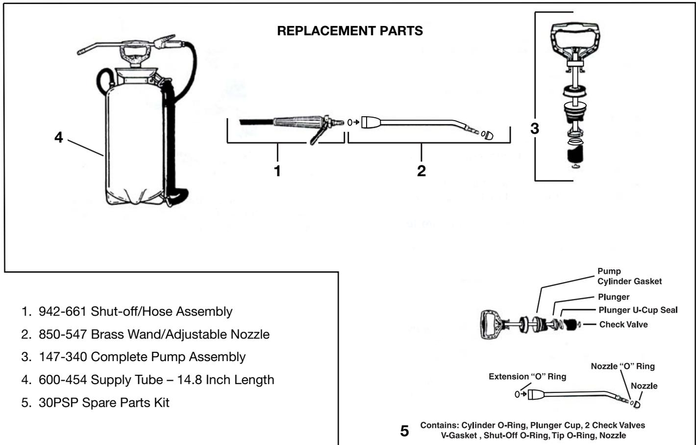
**IMPORTANT:** Replacement parts for No. 300P Sprayers made AFTER June 2018 are blue inked sprayer tanks. No. 300P Sprayers produced before June 2018 use black inked sprayer tanks and require different replacement parts – contact Nu-Calgon.
