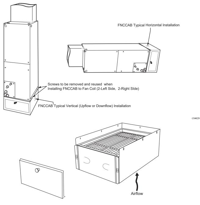
Install FILFNC Media Filter Cartridge in the FNCCAB Media Filter Cabinet.
