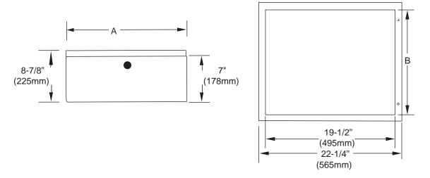
A09651 FNCCABXX0014 FNCCABXX0017 FNCCABXX0021 FNCCABXX0024 MODELS FNCCABXX0114 FNCCABXX0117 FNCCABXX0121 FNCCABXX0124 FNCCABXX0314 FNCCABXX0317 FNCCABXX0321 FNCCABXX0324 Airflow (CFM) Range 600-900 600-1350 600-2000 600-2200 14-5/16" (364mm) 17-5/8" (448mm) 21-1/8" (537mm) 24-5/8" (625mm) А В 11" (279mm) 14-11/32" (364mm) 17-7/8" (454mm) 21-11/32" (542mm) Shipping Weight 17 lb (7.7 kg) 17 lb-9 oz (8 kg) 19 lb-8 oz (8.8 kg) 23 lb (10.4 kg)
