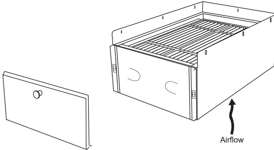
Install FILFNC Media Filter Cartridge in the FNCCAB Media Filter Cabinet.
