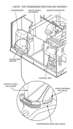
Secure heater to compressor so it straddles the compressor vertical shell weld seam and is positioned between the lower bearing pin weld and the comperssor base. To avoid wire damage, bend strap away from heater wires as shown.
