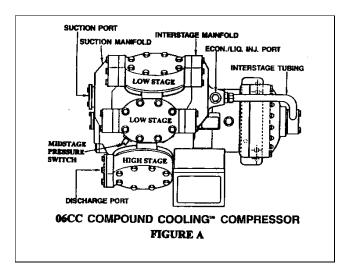
Important Note: On some older 06CC (50-99 cfms) when replacing the center bank valve plate there will be interference stemming from the addition of the relief valve to the replacement valve plate. To alleviate this interference problem remove the relief valve and install on opposite side of valve plate to act as a plug. Technician must confirm that the other low-stage valve plate has a pressure relief valve installed in the original orientation!
