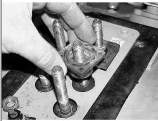
Install the flat washer, lock washer, and finger tighten the nut to secure the insulator block. Use the new nuts supplied with the kit.
