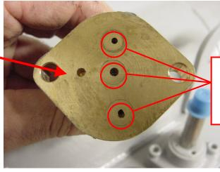
3 HOLES IN VALVE MUST LINE UP WITH HOLES ON COMP'R HOUSING
