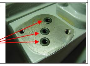
All Thunderbolt and 06Ns manufactured after the serial number listed above will use the 2TB1009 gasket. The solenoid valves are exactly the same however the compressor housings do not have the grooves for the o-rings and the gasket must be used.
