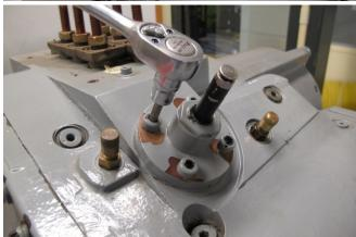
Install the o-rings into the grooves of the valve. Compressor oil or Parker Super-O-Lube can be used to help hold the o-rings inplace during reassembly.
