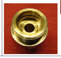
Re-install the Oil Filter Adaptor <u>without</u> the snap-ring and disc.
