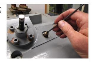
You can score the paint between the valve and the casing to provide a "clean break" when removing the valve. Remove the four socket head cap screws using a 6mm hex drive. It is helpful to strike the cap screws using a hammer and drift. This will make it easier to remove the screws. Lift the valve from the casing, being careful not to allow any dirt or paint chips to fall into the holes.
