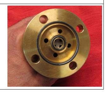
Install new valve using the new orings and socket head cap screws. Torque screws to:
