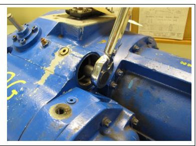
Install the oil filter. Replace the o-ring on the filter access plug by sliding the new o-ring over the back side of the plug. Installing the o-ring over the threads can cut the o-ring causing leaks. Lubricate the o-ring with compressor oil or Parker Super-O-Lube. Torque the access plug to:
