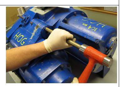
Remove the oil filter by pulling it off the adapter. It's a good idea to replace the filter at this time. Many filters are damaged during removal.
