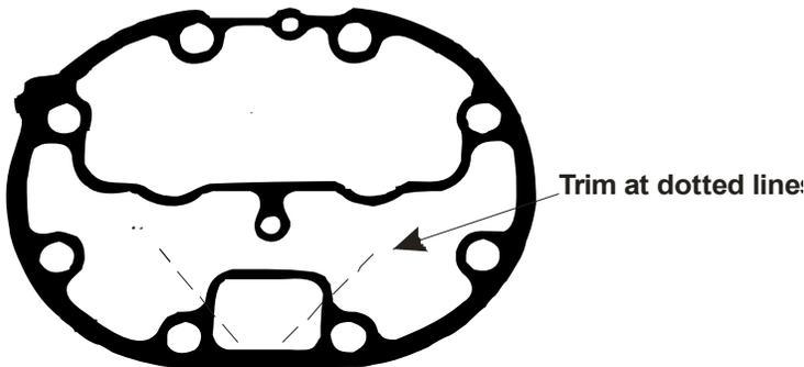
The gasket pictured above (06EA503314 HGBP) is included in this kit. When this gasket is used on a sidebank non-unloading cylinder head, trim the crossover port as indicated.
