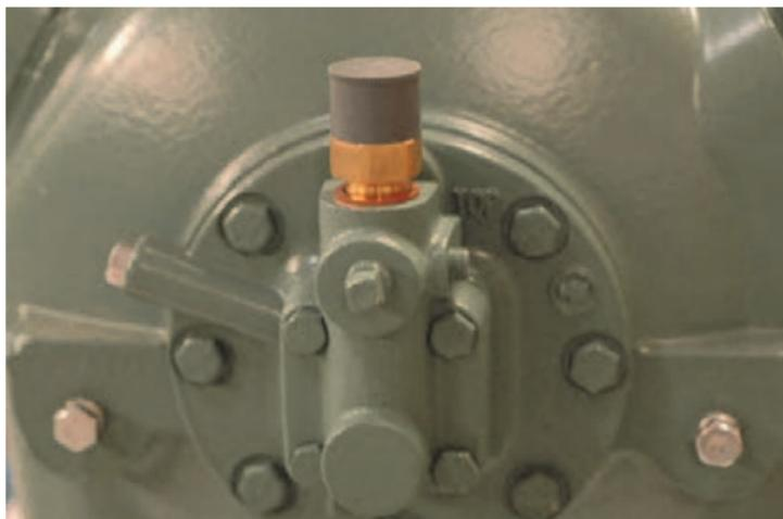
**Fig. 20: Sensor del interruptor OPSS instalado**
