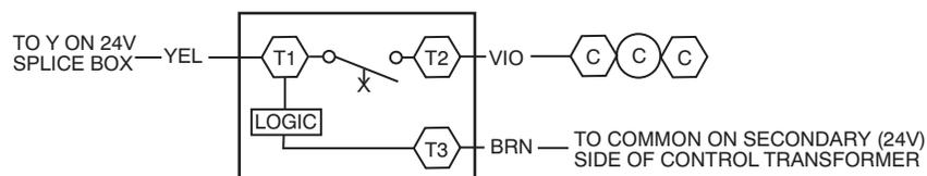
Fig. 4 - Time Guard II Device Wiring Diagram - 1-1/2 to 5 Ton Gas Heat/Electric Cooling, Electric Heat/Electric Cooling Units Without Safety Device
