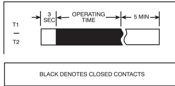
Fig. 2 - Time Guard II Device Sequence Chart
