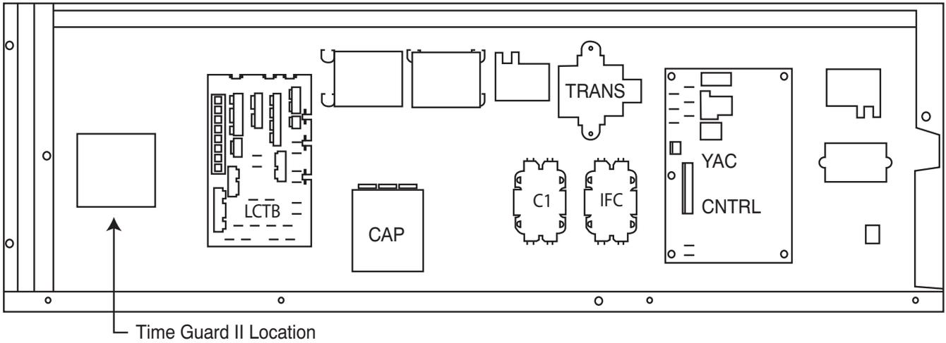
**Fig. 7 - Time Guard II Device Mounting on 3 to 12-1/2 Ton Gas Heat/Electric Cooling, Electric Heat/Electric Cooling Units with R-410A Refrigerant**
