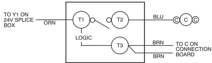
Fig. 11 - Wire Connections, 6 to 10 Ton Condensing Units
