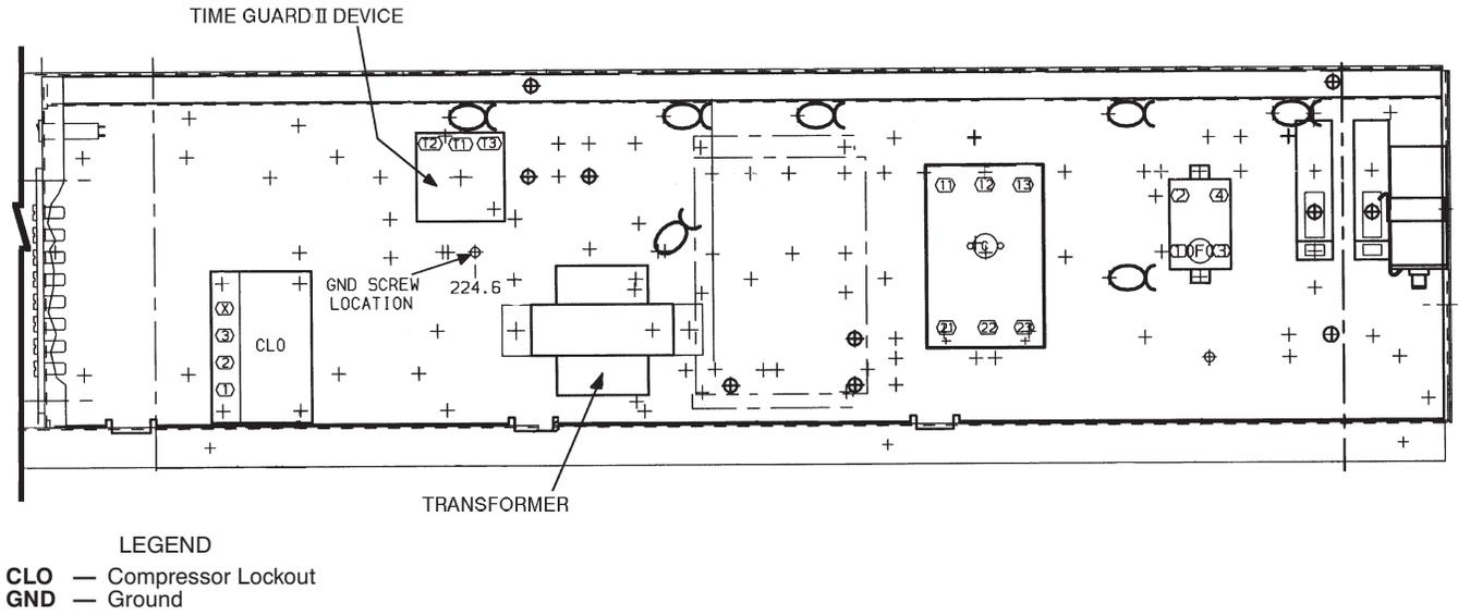
Fig. 10 - Time Guard II Device Mounted on 6 to 10 Ton Condensing Units
