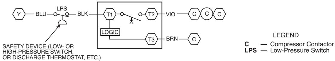
**Fig. 5 - Time Guard II Device Wiring Diagram - 1-1/2 to 5 Ton Gas Heat/Electric Cooling, Electric Heat/Electric Cooling Units With Safety Device(s)**
