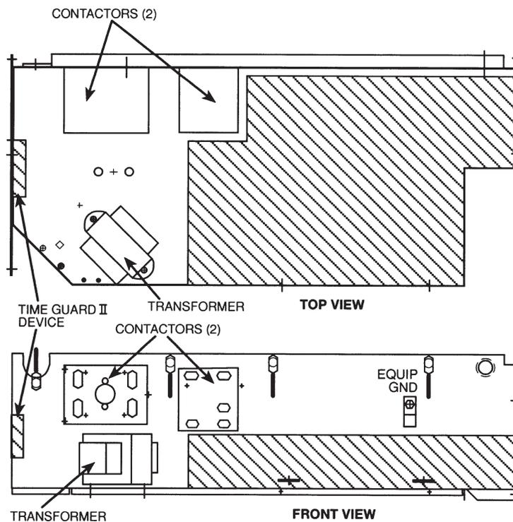
Fig. 3 - Time Guard II Device Mounted on 1-1/2 to 5 Ton Small Packaged Gas Heat/Electric Cooling, Electric Heat/Electric Cooling Units
