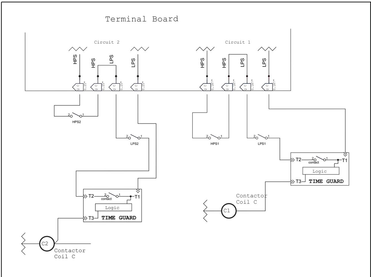
**Fig. 8 - Wiring Diagram, Time Guard II Device for 3 to 12-1/2 Ton Units (1 and 2 Compressor Systems) with R-410A Refrigerant**
