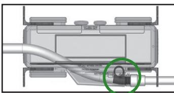
**Horizontal drain for restricted height applications over doors and windows, showing top access for lineset.**
