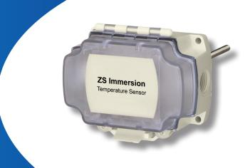
The Carrier communicating ZS immersion sensors line is designed to monitor water temperature in pipe applications. The sensor is potted inside a 1/4" stainless steel probe with a thermally conductive compound. All immersion units are mounted in a thermowell and have etched Teflon lead-wires and double encapsulated sensors to create a watertight package that can withstand a wide range of humidity and condensation.
