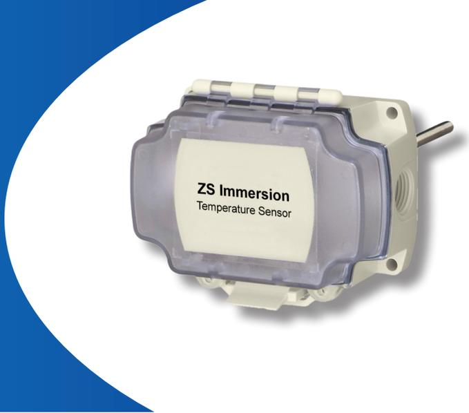
The Carrier communicating ZS immersion sensors line is designed to monitor water temperature in pipe applications. The sensor is potted inside a 1/4" stainless steel probe with a thermally conductive compound. All immersion units are mounted in a thermowell and have etched Teflon® lead-wires and double encapsulated sensors to create a watertight package that can withstand a wide range of humidity and condensation.
