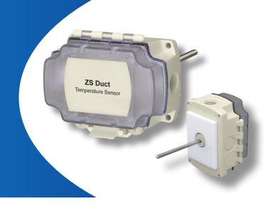
The Carrier communicating ZS duct sensors line is designed to measure the air temperature and/or humidity in ductwork. All duct sensors feature closed cell foam to seal the insertion hole and to absorb vibration. Mounting tabs allow for easy installation onto the wall of the duct. The units are built to withstand high humidity and condensation environments.
