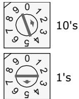
**! CAUTION** The factory default setting is **00** and must be changed to successfully install your UPC Open.
