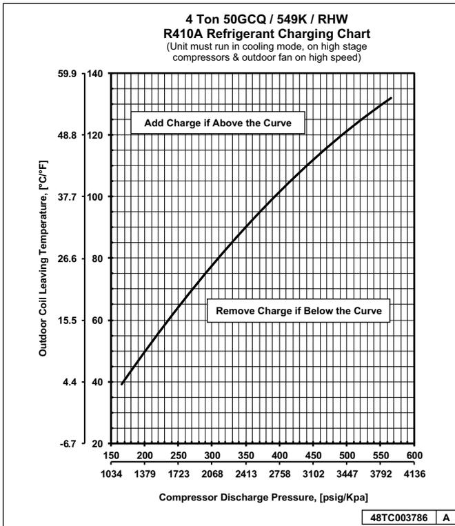
Fig. 23 — Cooling Charging Chart - 4 Ton
