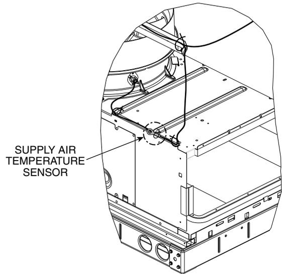
**Fig. 59 — Supply Air Sensor Location**
