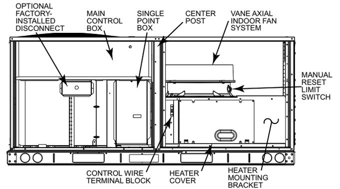
Fig. 34 — Typical Component Location
