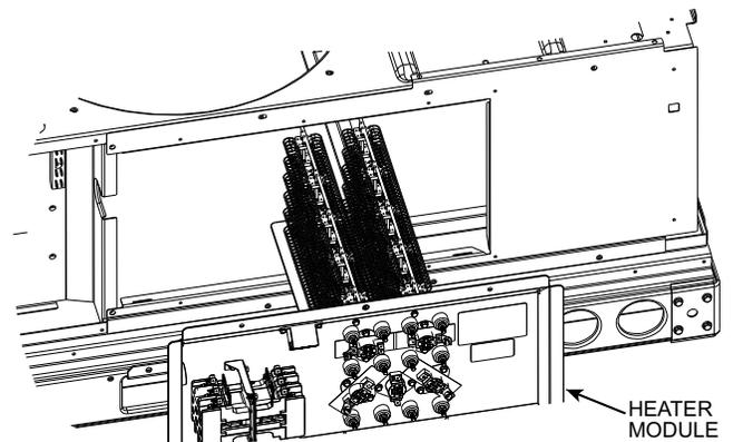
Fig. 35 — Typical Module Installation
