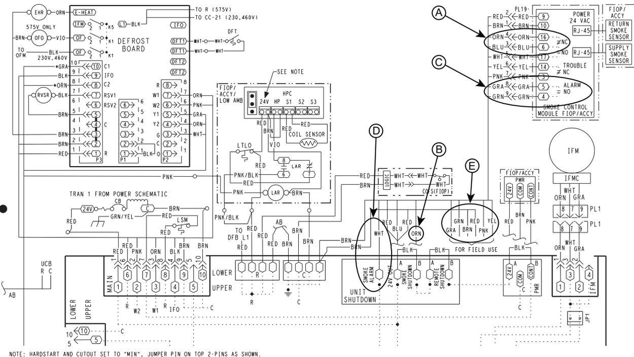
**Fig. 46 — Typical Smoke Detector System Wiring**
