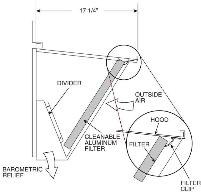
**Fig. 3 — Filter Installation**
