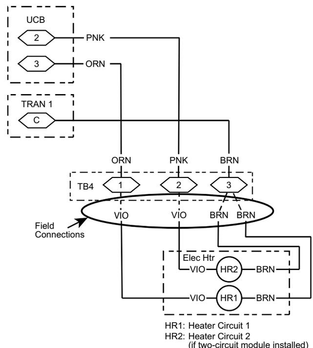
**Fig. 38 — Accessory Electric Heater Control Connections**
