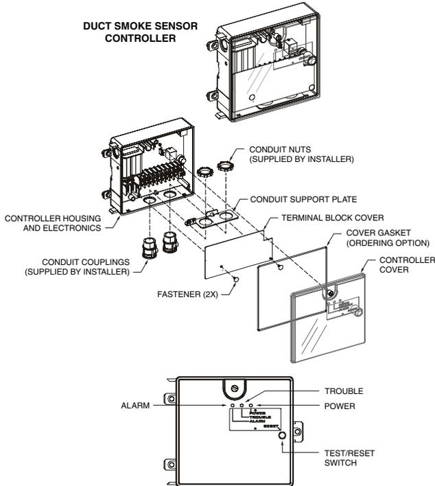
**Fig. 39 — Controller Assembly**
