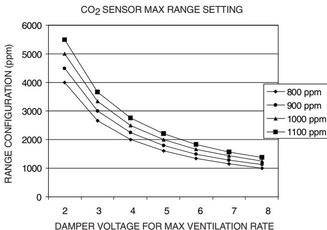
**Fig. 65 — CO<sub>2</sub> Sensor Maximum Range Settings**
