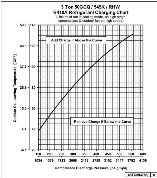
Fig. 22 — Cooling Charging Chart - 3 Ton
