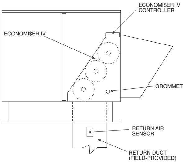
**Fig. 62 — Return Air Temperature or Enthalpy Sensor Mounting Location**
