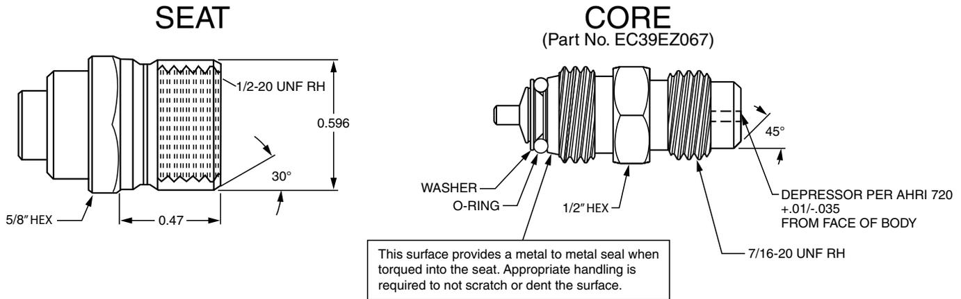
Fig. 21 — CoreMax<sup>1</sup> Access Port Assembly
