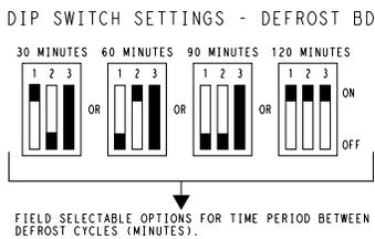
Fig. 32 — DIP Switch Settings - Defrost Board
