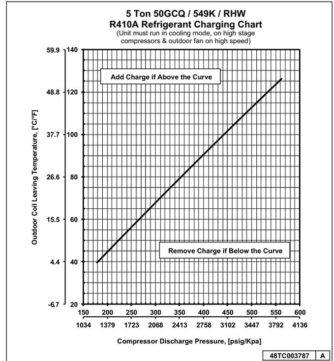
Fig. 24 — Cooling Charging Chart - 5 Ton
