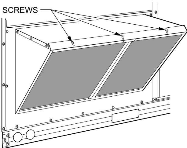
**Fig. 4 — Screens Installed on Outdoor-Air Hood**
