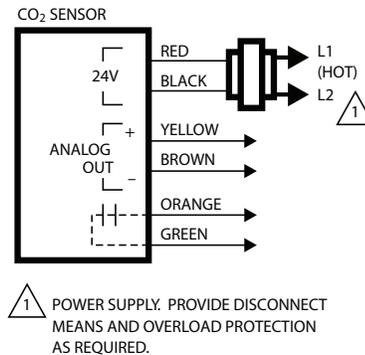
**Fig. 70 — CO<sub>2</sub> Sensor Wiring**
