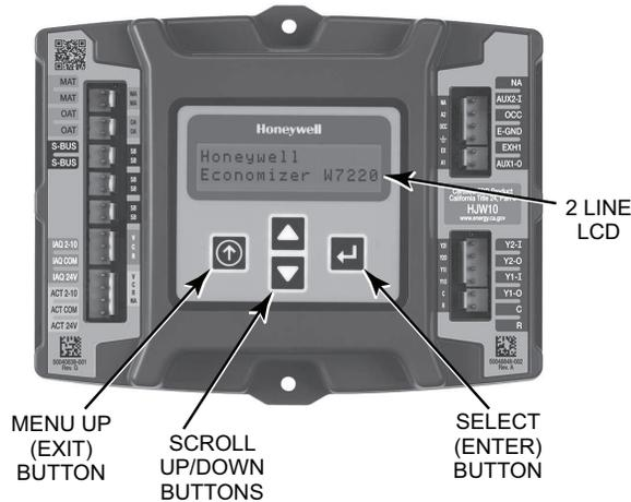
**Fig. 71 — W7220 Controller Navigation Buttons**
