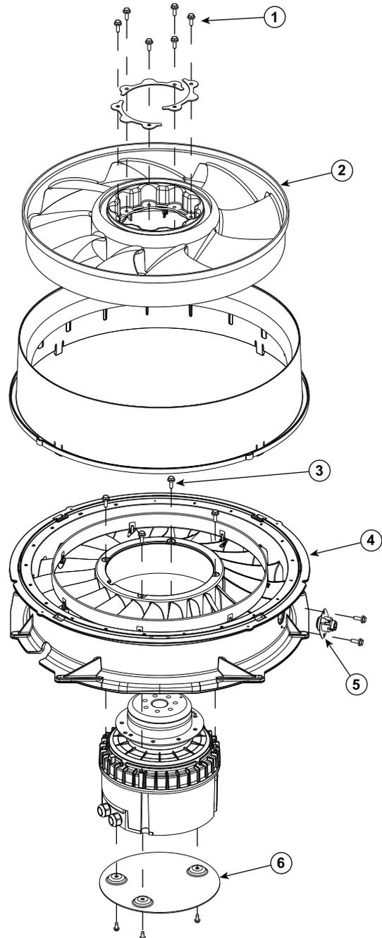
**Fig. 12 — Disassembling Motor and Fan Assembly**
