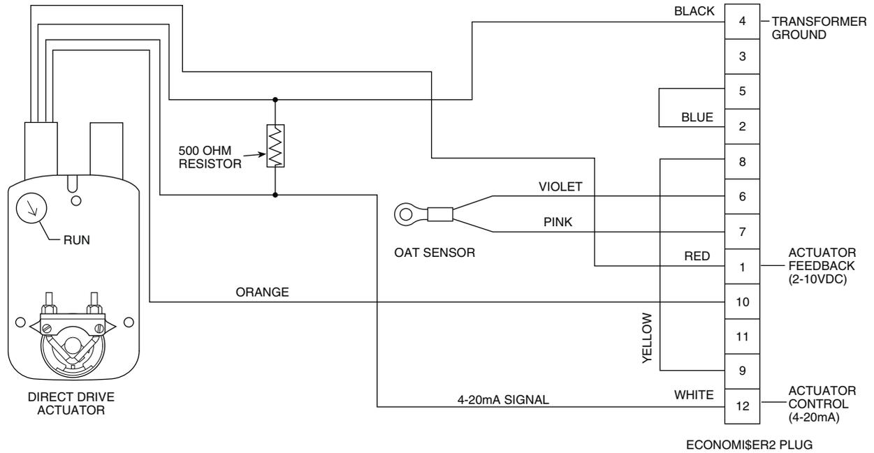
**Fig. 55 — EconoMi\$er2 with 4 to 20 mA Control Wiring**
