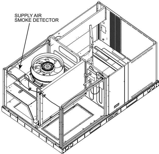
**Fig. 41 — Typical Supply Air Smoke Detector Sensor Location**
