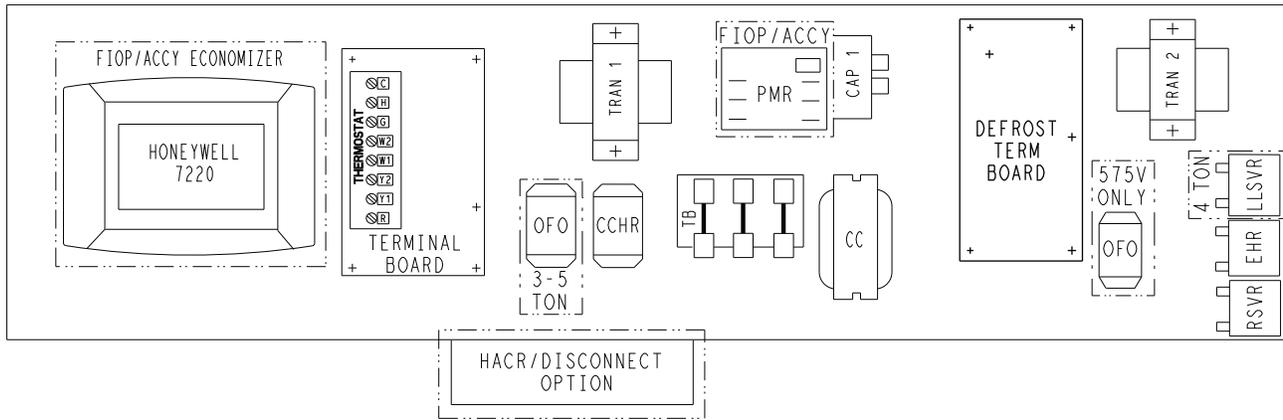
**Fig. 31 — Defrost Control Board Location - 50GCQ 04-06 Electro-Mechanical Units**
