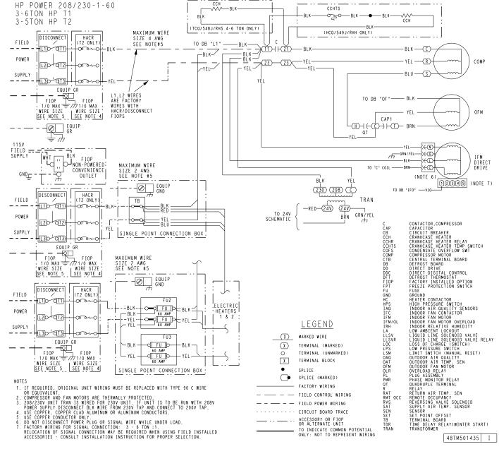
Fig. 43 — Electro-Mechanical Power Wiring: 208/230-1-60
