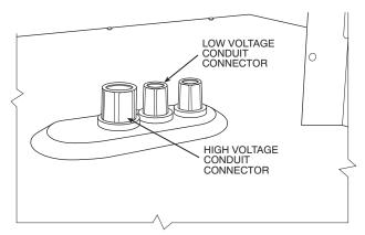
Fig. 29 — Thru-Base Connection Fittings (Units Built Prior to 4/15/2019)
