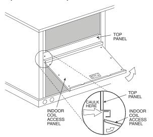
Fig. 16 — Indoor Coil Access Panel Relocation
