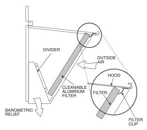
Fig. 18 — Economizer Filter Installation
