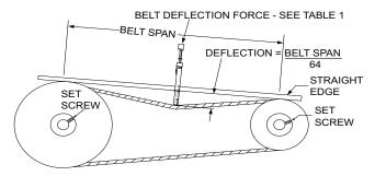
TORQUE ALL SHEAVE SET SCREWS TO 110-130 in. lbs TABLE 1
