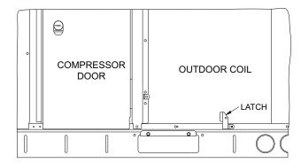
Fig. 19 — Compressor Door Latch Location
