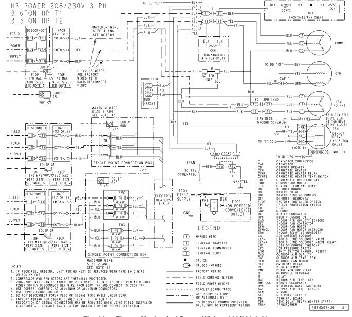
Fig. 44 — Electro-Mechanical Power Wiring: 208/230-3-60
