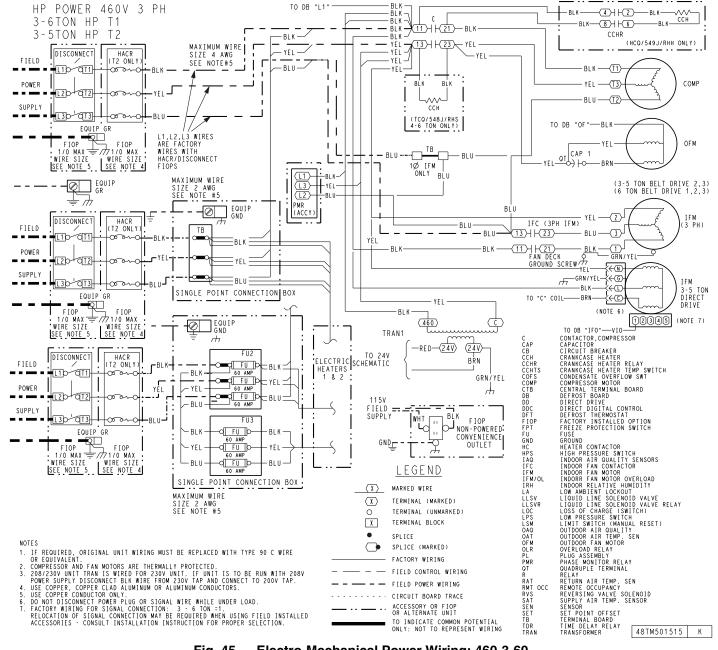
Fig. 45 — Electro-Mechanical Power Wiring: 460-3-60
