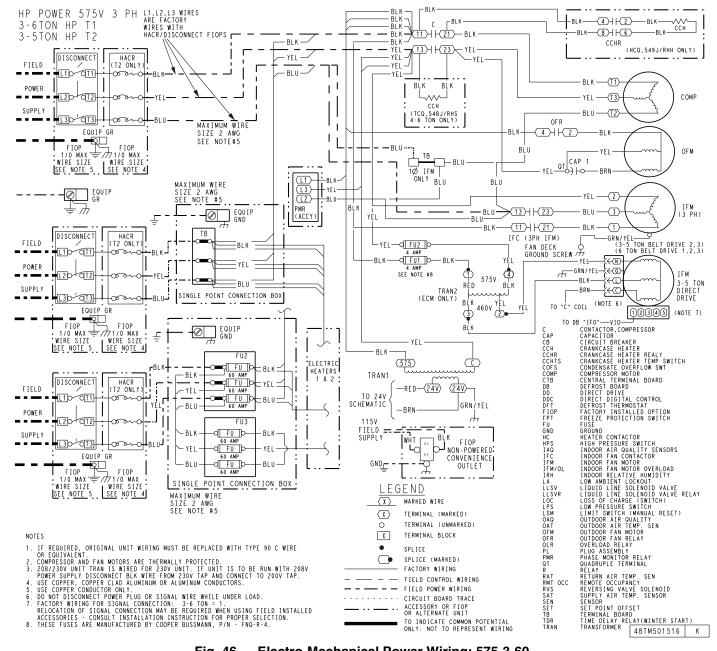
Fig. 46 — Electro-Mechanical Power Wiring: 575-3-60
