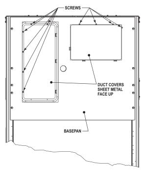
Fig. 12 — Horizontal Duct Panels In Place
