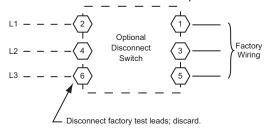
Fig. 23 — Power Wiring Connections
