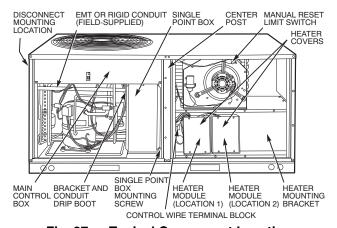
Fig. 37 — Typical Component Location
