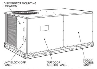
Fig. 36 — Typical Access Panel Location (3-6 Ton)
