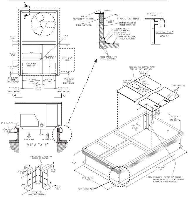
Fig. 7 — Roof Curb Details
