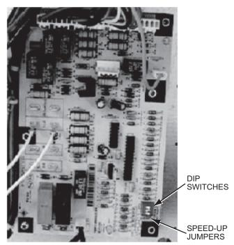
Fig. 33 — Defrost Control Board Arrangement
