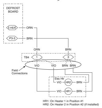
Fig. 40 — Accessory Electric Heater Control Connections
