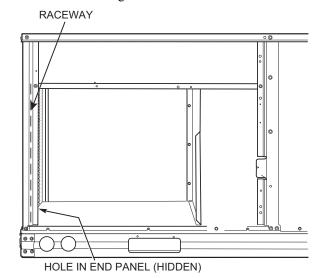
Fig. 32 — Field Control Wiring Raceway
