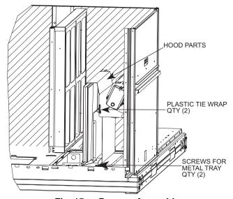
Fig. 15 — Damper Assembly
