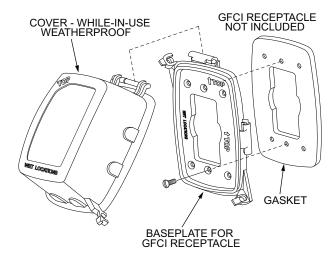
Fig. 25 — Weatherproof Cover Installation
