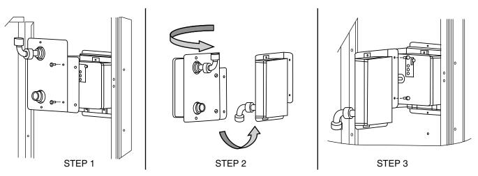
Fig. 57 — Completing Installation of Return Air Smoke Sensor
