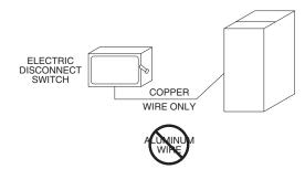
Fig. 22 — Disconnect Switch and Unit
