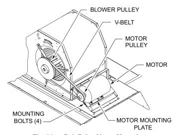
Fig. 60 — Belt Drive Motor Mounting
