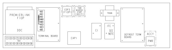
NOTE: IFC ONLY FOR 3Ø IFM, IFC NOT REQUIRED FOR DIRECT DRIVE MOTOR OPTION.
