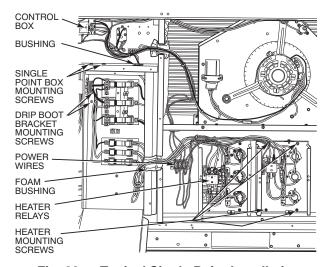
Fig. 39 — Typical Single Point Installation
