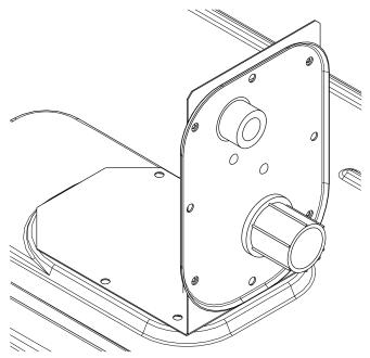
Fig. 28 — Thru-the-Base Fitting Assembly (Shown in Shipping Position)
