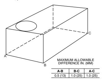
Fig. 8 — Unit Leveling Tolerances
