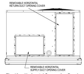
Fig. 10 — Horizontal Conversion Panels
