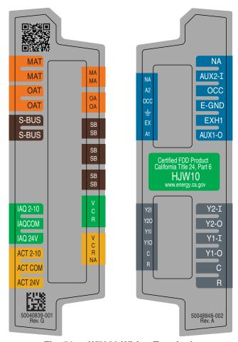
Fig. 51 — W7220 Wiring Terminals
