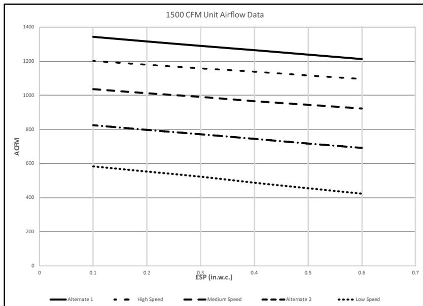
Fig. 5 – Static Pressure - 015 Size
