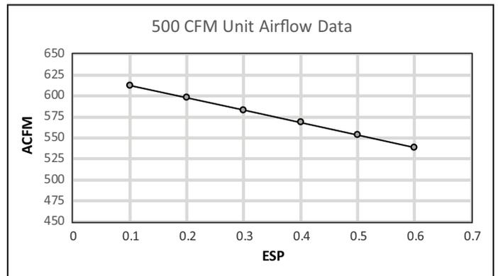
**Fig. 3 – Static Pressure - 005 Size**
