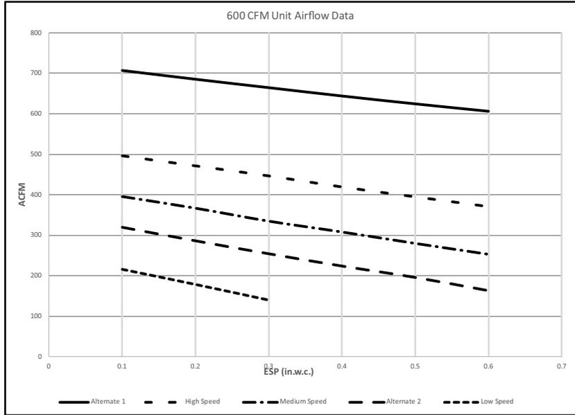
Fig. 4 – Static Pressure - 006 Size
