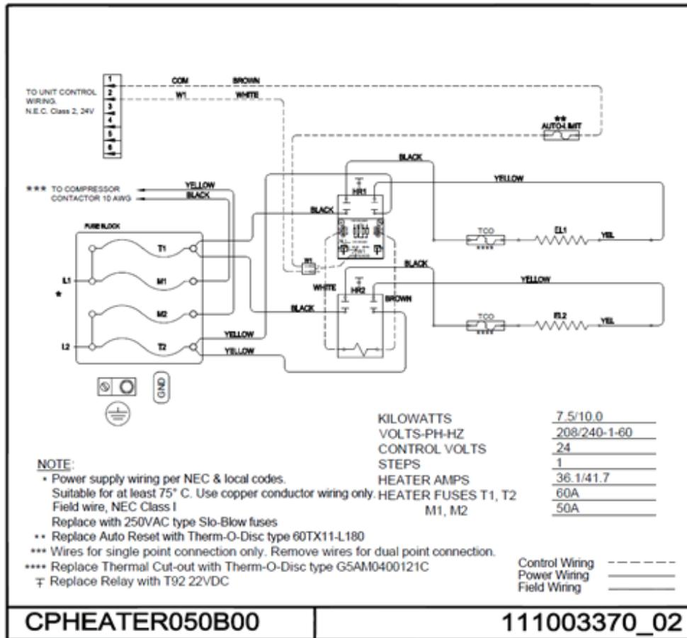
**Fig. 14 – CPHEATER52B00 Wiring Diagram**
