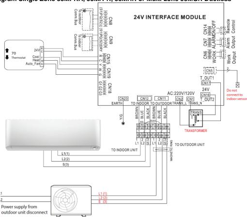
2. Wiring Diagram Single Zone 38MBR Ductless
