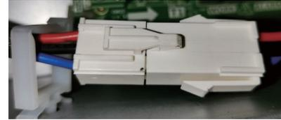
**Fig. 9 — Insert the white plug**
