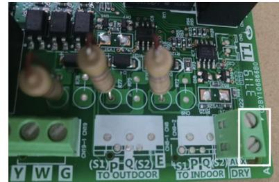
**Fig. 10 — Connect the auxiliary heat wires**
