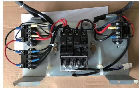
**Fig. 11 — Choose the power cord installation location**
