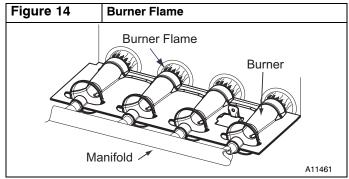
**NOTE**: Gas valve regulator seal cap MUST be in place when checking input rate. When correct input is obtained, main burner flame should be clear blue, almost transparent (See **Figure 14**). Be sure regulator seal cap is in place when finished.
