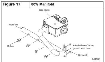
**NOTE**: Use a back-up wrench on the gas valve to prevent the valve from rotating on the manifold or damaging the mounting to the burner box. (See **Figure 16** & **Figure 17**)
