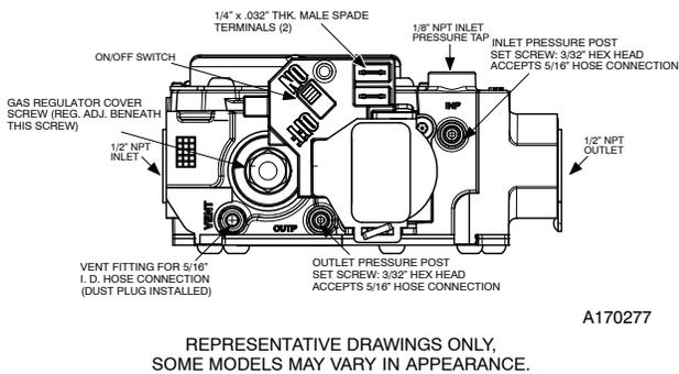
**Fig. 16 – Manifold Pressure Adjusting Key**
