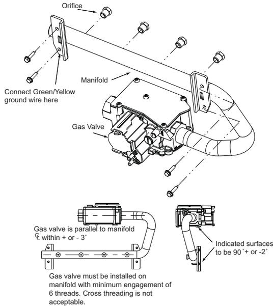
**Fig. 4 – Manifold Assembly**
