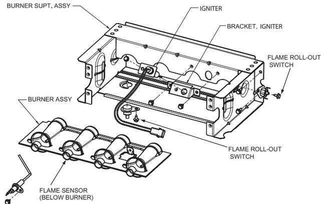
**Fig. 5 – Burner Assembly**
