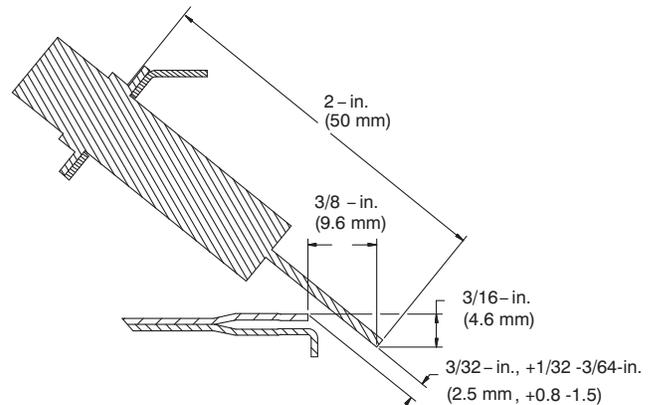
Fig. 10 – Igniter Position – Side View
