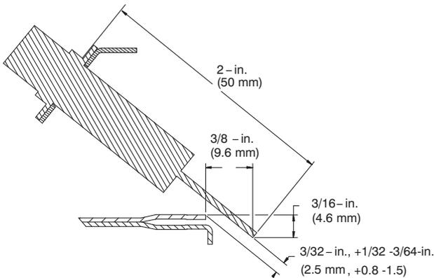
Fig. 9 - Igniter Position - Side View
