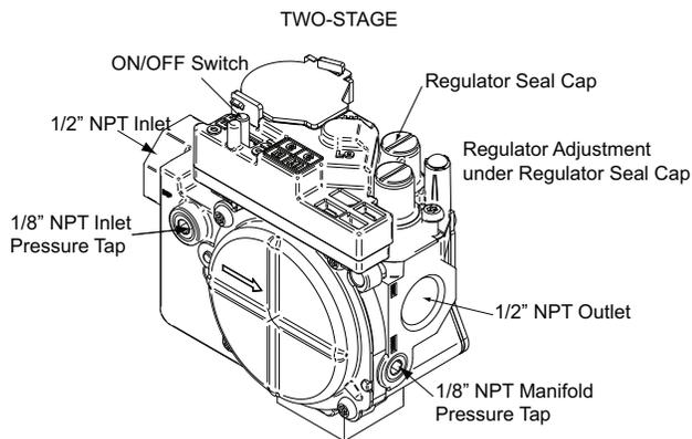
**Automatic Gas Valve (Two-Stage) without Tower Pressure Ports**
