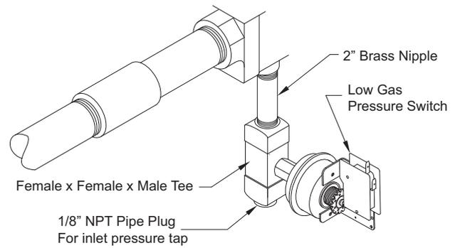
**Fig. 30 - 80% Low Gas Pressure Switch**
