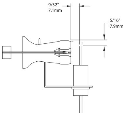
**Fig. 25 - Igniter Position - Side View**
