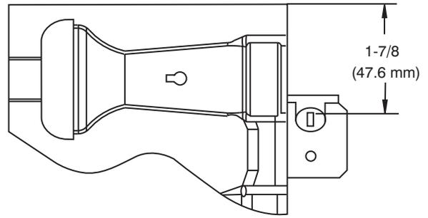
**Fig. 26 - Igniter Position - Top View**
