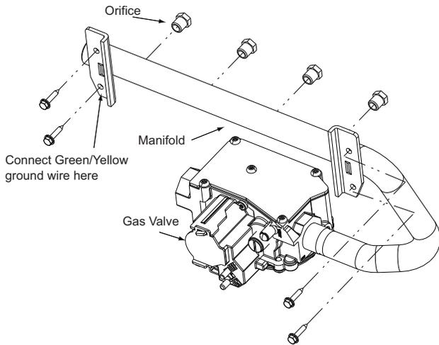
**Fig. 2 - Manifold Assembly**
