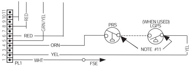
Fig. 31 - 80% Pressure Switch Wiring
