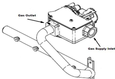
**Fig 1- Gas Valve/ Manifold Assembly****Step 4 -- Installation of low gas pressure switch (propane units only)**
