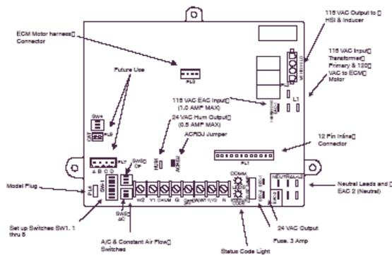
**Fig. 6 - Variable Speed Furnace Control**
