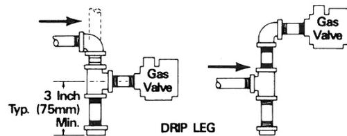
8. **DO NOT** insert any object other than suitable pipe or tubing in the inlet or outlet of this control. Internal damage may occur and result in a hazardous condition. A backup wrench should only be used on the wrench boss provided for this purpose (see drawing), never on body of the control, as this could distort the casting. **NOTE:** Do not overtighten any pipe connections, as this could crack the valve body. A valve with a cracked valve body will not be warranted.
