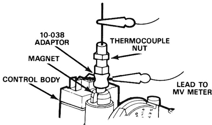
5. Check closed circuit thermocouple output. If less than eight millivolts, replace with Robertshaw 1970 or 1980 series thermocouple.
