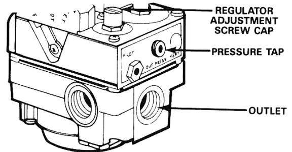
1. Manometer or gauge attachment may be accomplished at pressure tap plug.
