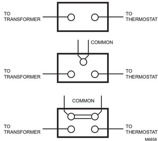
Fig. 6. Wiring connections on standing pilot gas controls.
