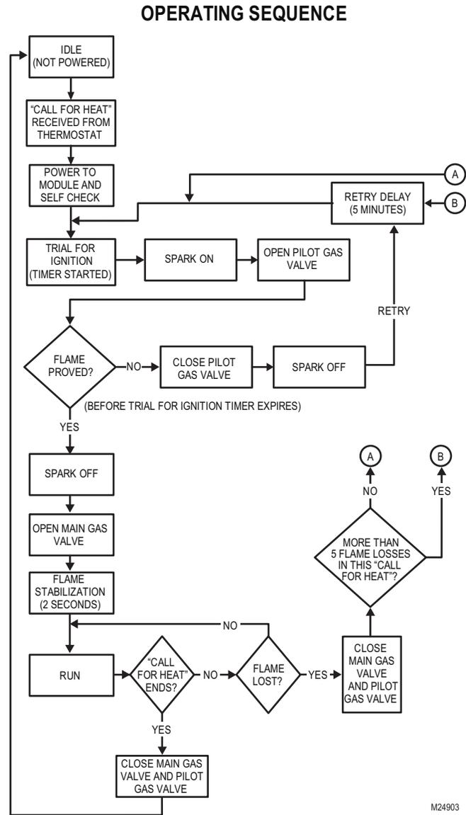
Fig. 19. Normal operating sequence without vent damper.
