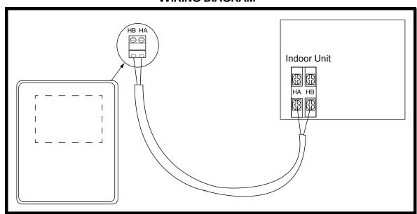
Use wire size 20AWG to 16AWG stranded, shielded, 2-core.
