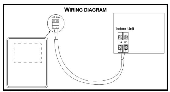
Use wire size 18AWG stranded, shielded, 2-core
