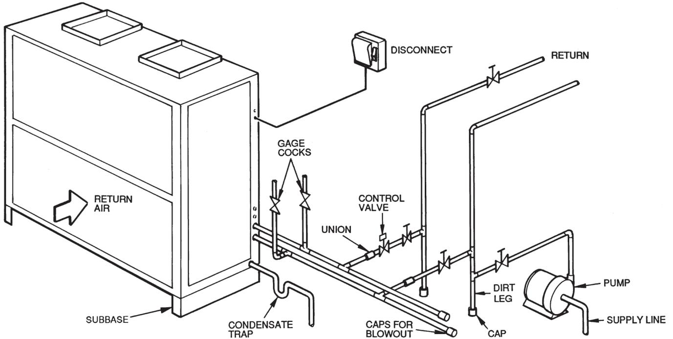
**Fig. 12 - Typical 40RUS Chilled Water Piping**
