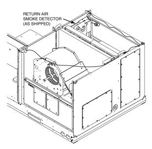
Fig. 56 — Return Air Smoke Detector, Shipping Position
