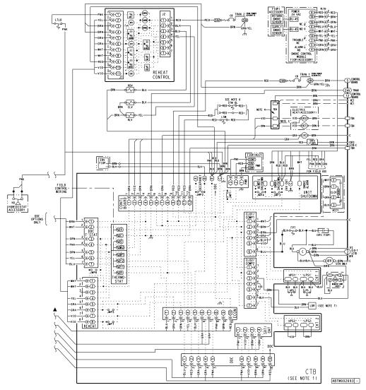
Fig. 40 — Typical Humidi-MiZer® Adaptive Dehumidification System Humidistat Wiring
