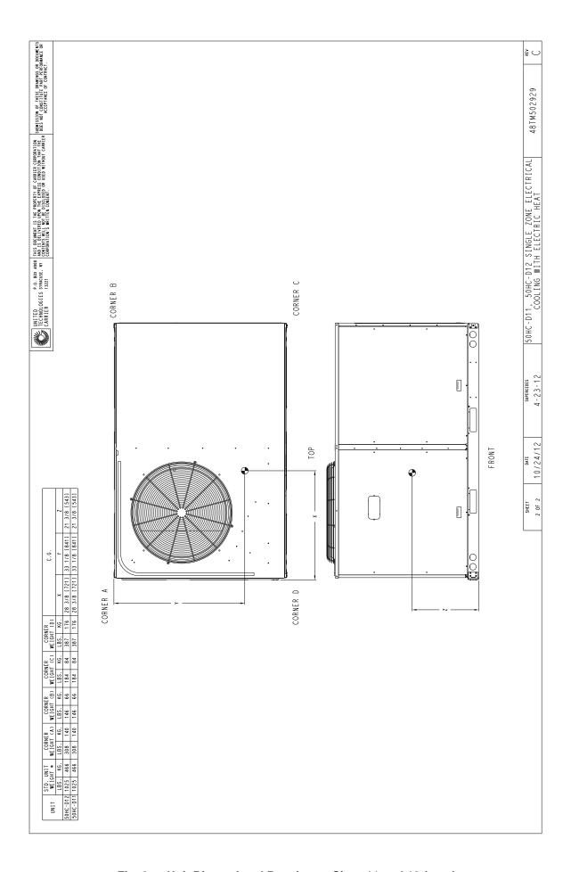
Fig. 3 — Unit Dimensional Drawing — Sizes 11 and 12 (cont)
