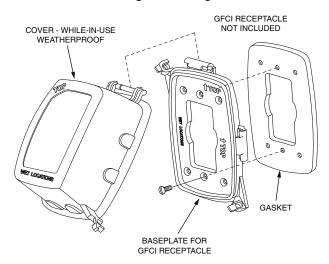
Fig. 27 — Weatherproof Cover Installation
