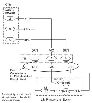
Fig. 37 — Optional or Accessory Electric Heater Control Connections for CRHEATER128B00-129B00 Only
