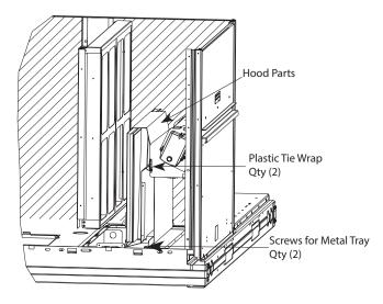
Fig. 12 — Economizer and Two-Position Damper Hood Parts Location
