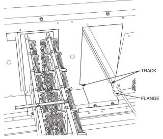
Fig. 34 — Typical Module Installation
