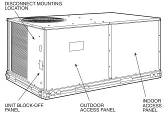
Fig. 32 — Typical Access Panel Location
