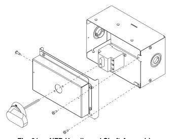
Fig. 21 — NFD Handle and Shaft Assembly
