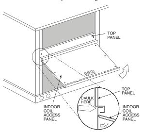
Fig. 13 — Indoor Coil Access Panel Relocation
