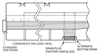
Fig. 16 — Condensate Drain Pan (Side View)
