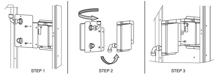
Fig. 57 — Completing Installation of Return Air Smoke Sensor
