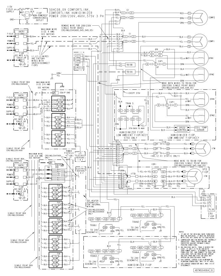
Fig. 45 — Typical 50HC ComfortLink Control Power Wiring Diagram with Humidi-MiZer® System (208/230V, 460V-3 Ph-60 Hz shown)
