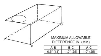
Fig. 5 — Unit Leveling Tolerances
