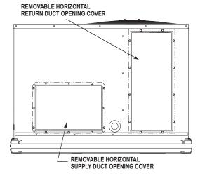
Fig. 8 — Horizontal Conversion Panels
