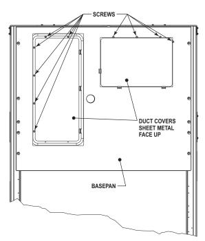
Fig. 10 — Horizontal Duct Panels In Place
