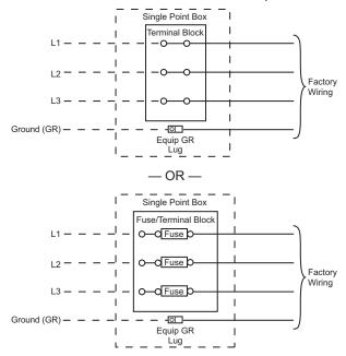
Fig. 18 — Power Wiring Connections
