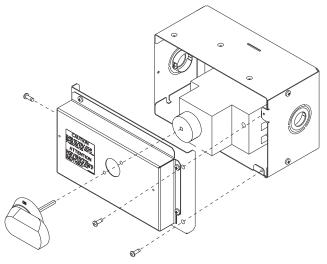
Fig. 23 — HACR Handle and Shaft Assembly
