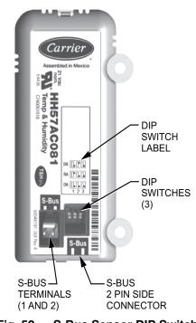
Fig. 52 — S-Bus Sensor DIP Switches
