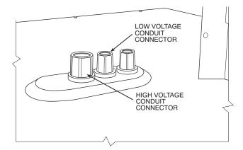
Fig. 29 — Thru-Base Connection Fittings
