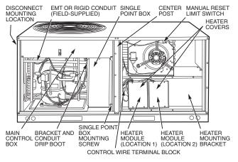
Fig. 33 — Typical Component Location
