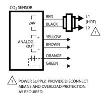
Fig. 53 — CO<sub>2</sub> Sensor Wiring
