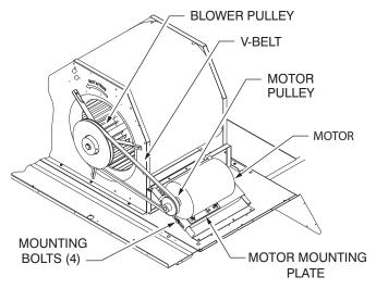
Fig. 60 — Belt Drive Motor Mounting
