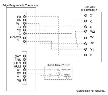
Fig. 41 — Typical Rooftop Unit with Humidi-MiZer® Adaptive Dehumidification System with Edge® Pro Thermidistat Device
