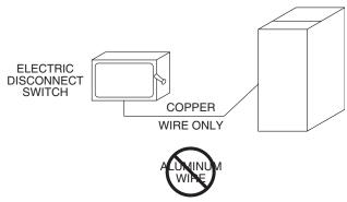
Fig. 19 — Disconnect Switch and Unit
