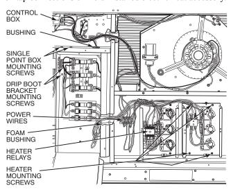
Fig. 35 — Typical Single Point Installation
