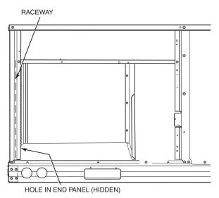
Fig. 31 — Field Control Wiring Raceway
