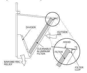
Fig. 15 — Economizer Filter Installation
