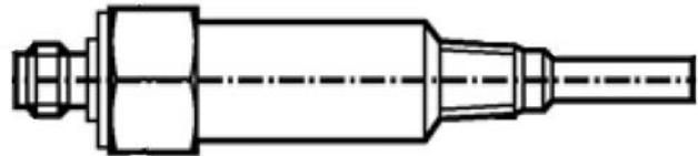
**Fig. 48 — Thermal Flow Sensor**
