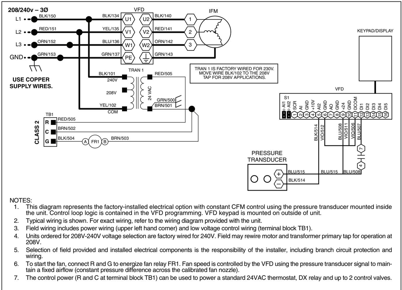
**Fig. 89 — Control Option “D,” Constant CFM Control Typical Wiring Diagram**
