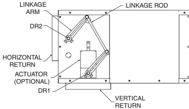
**Fig. 57 — Linkage Assembly Front View
