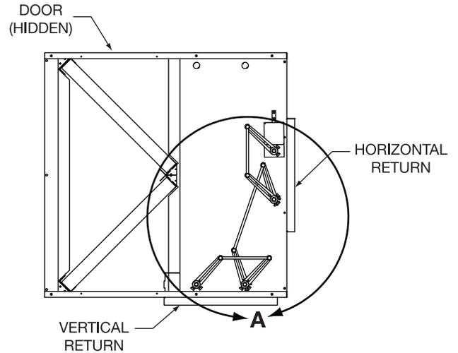
**Fig. 59 — Linkage Assembly Front View
