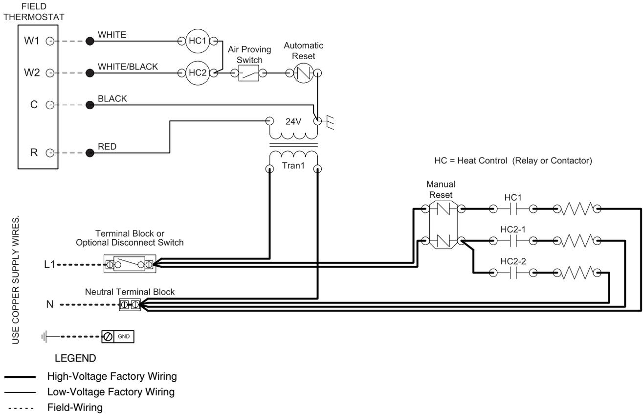
**Fig. 80 — Electric Heat Wiring Schematic, Dual Point Power (3 Elements), 277V, Single Phase, 11 to 13 kW**
