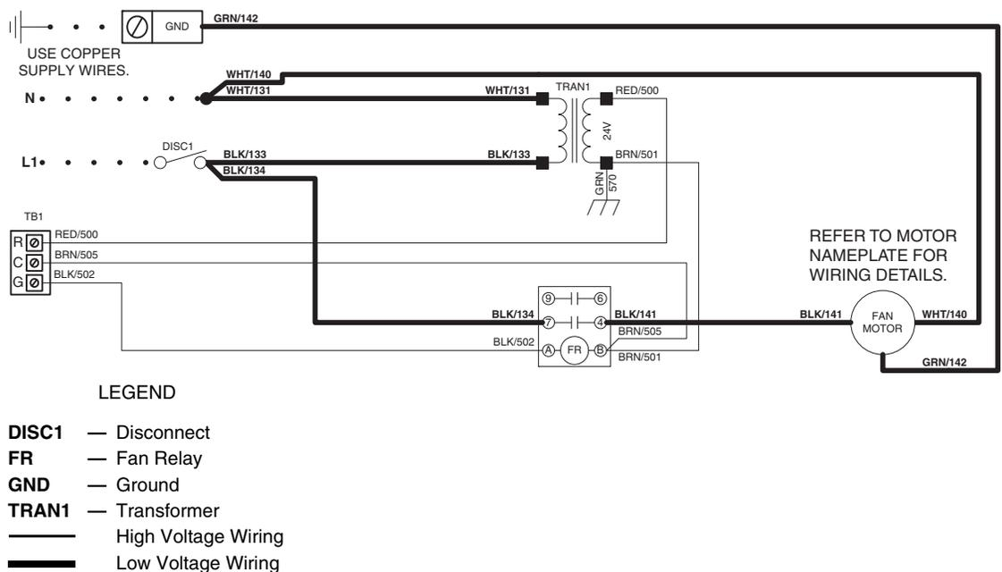
**Fig. 94 — Typical Wiring Diagram, Single-Phase Relay Control**
