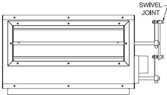
**Fig. 58 — Linkage Assembly Side View
