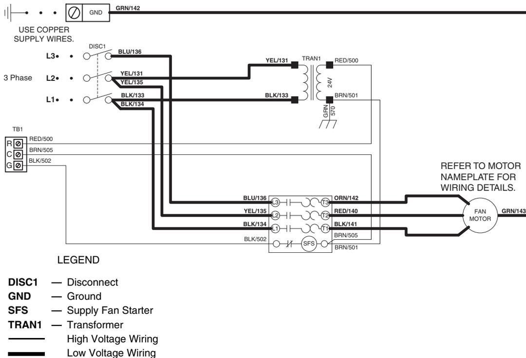
**Fig. 96 — Typical Wiring Diagram, Three-Phase Starter Control**
