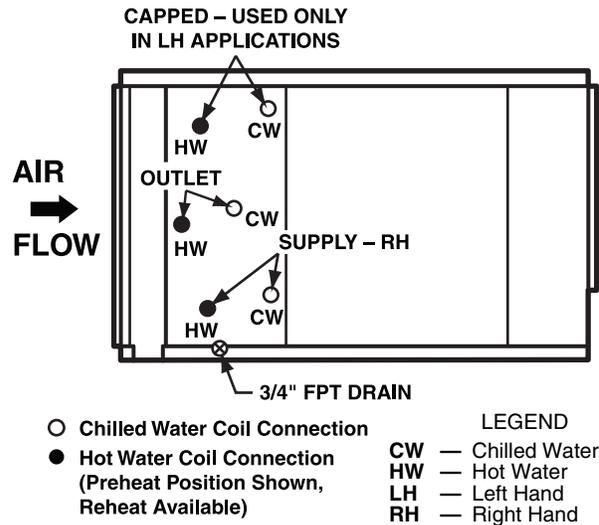
Fig. 66 — Water Coil Connection
