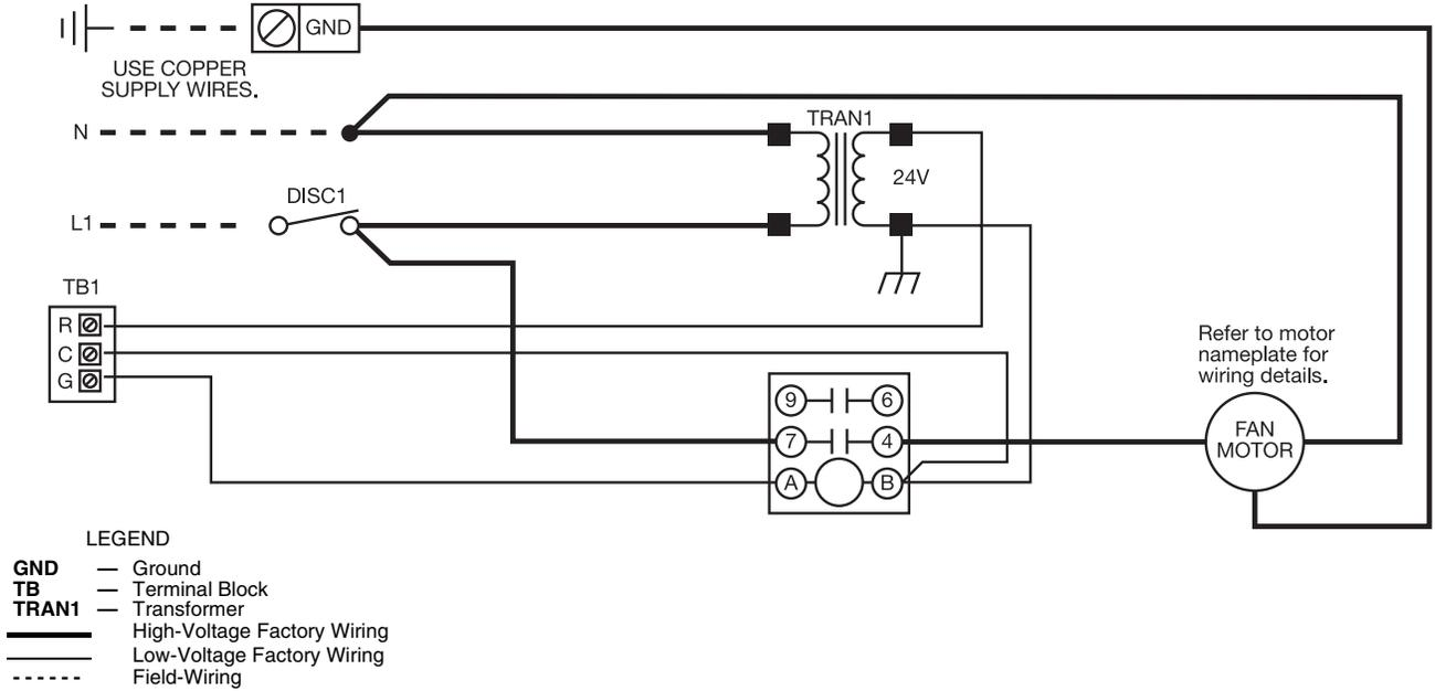
**Fig. 84 — Single-Phase Motor Start/Stop Station Wiring Diagram**
