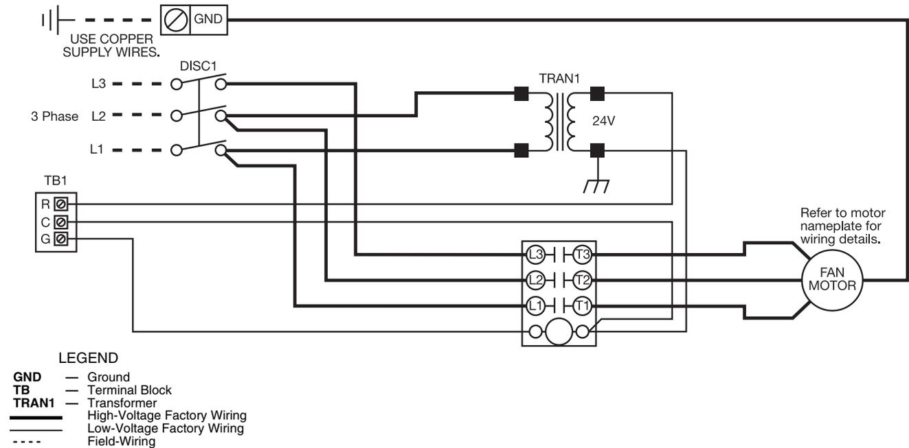
**Fig. 85 — 3-Phase Motor Start/Stop Station Wiring Diagram**
