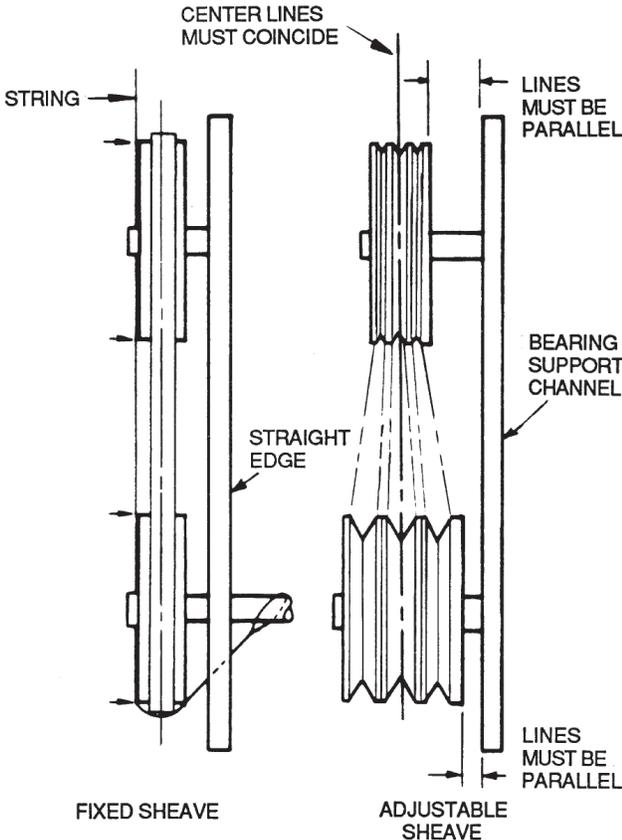
**Fig. 64 — Sheave Alignment**
