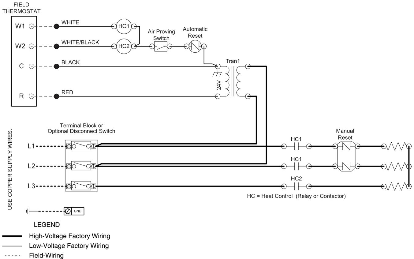
**Fig. 82 — Electric Heat Wiring Schematic, Dual Point Power (Star Wiring), 240V 3-Phase 1 to 10 kW and 480V 3-Phase 2 to 20 kW**
