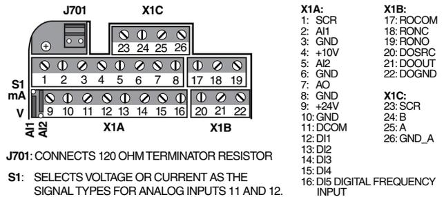
J701: CONNECTS 120 OHM TERMINATOR RESISTOR
