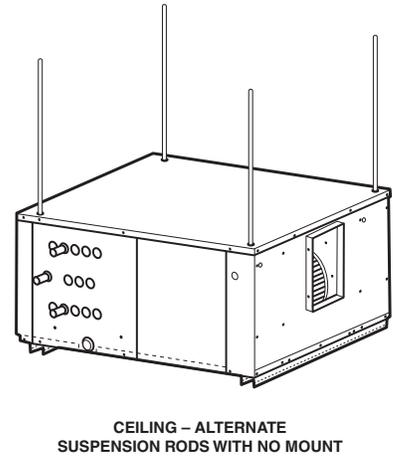
**Fig. 23 — Unit Suspension**
