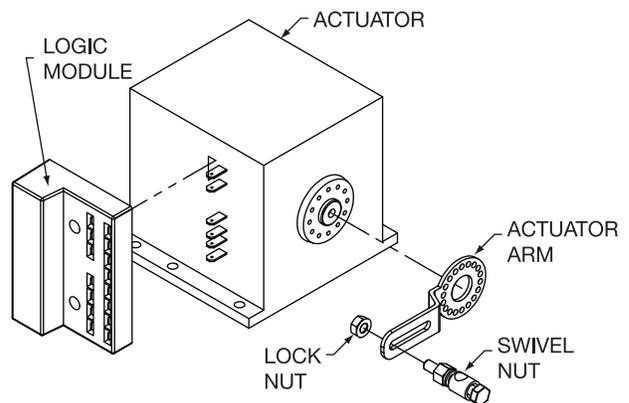
**Fig. 47 — Actuator Assembly**
