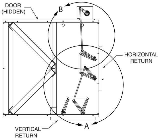
**Fig. 49 — Actuator Installation Front View**
