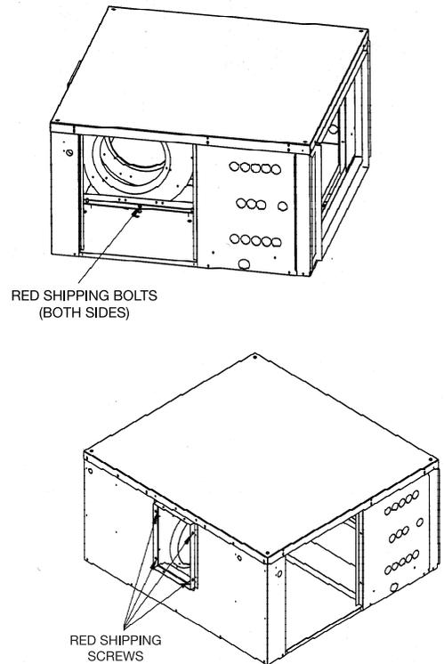
**Fig. 22 — Shipping Bolt and Screw Removal**
