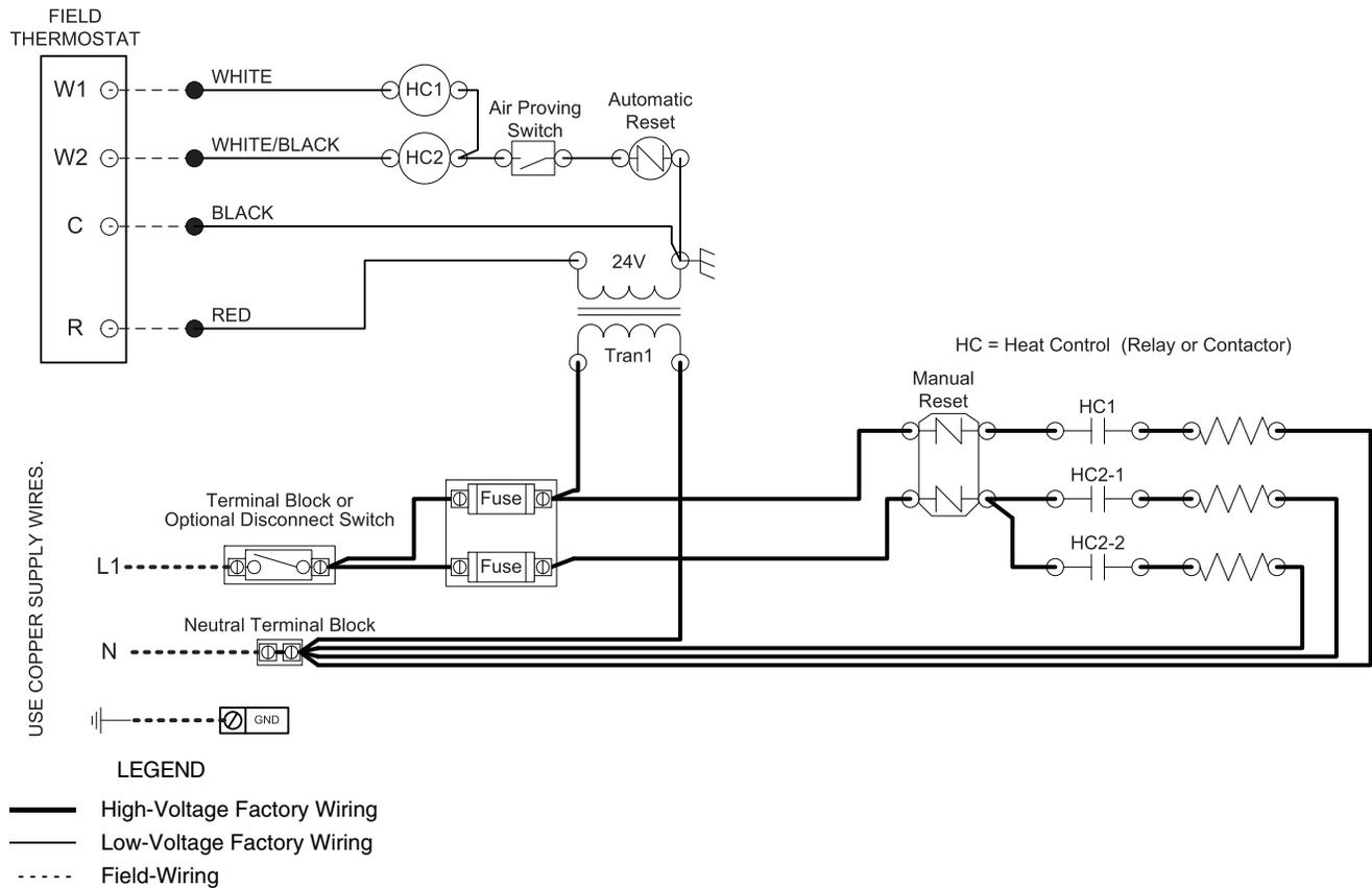
**Fig. 81 — Electric Heat Wiring Schematic, Dual Point Power (3 Elements), 277V, Single Phase, 14 to 17 kW**
