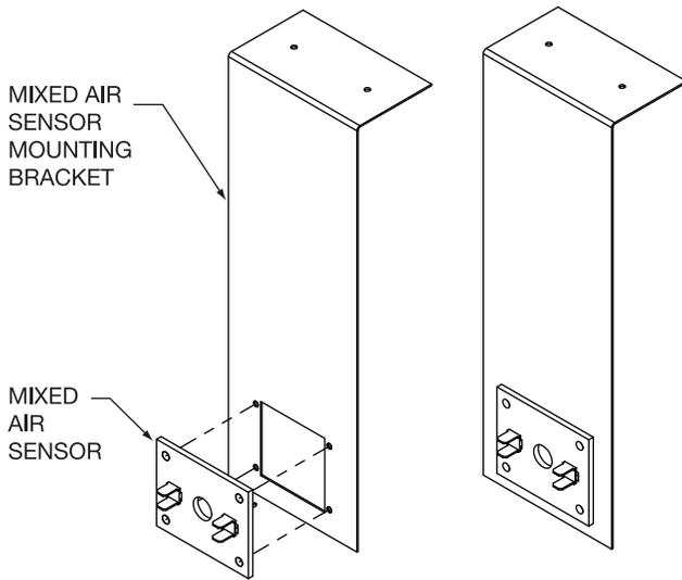
**Fig. 53 — Mixed Air Sensor Bracket**
