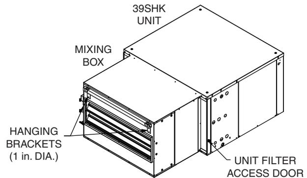
**Fig. 56 — Installing Mixing Box**
