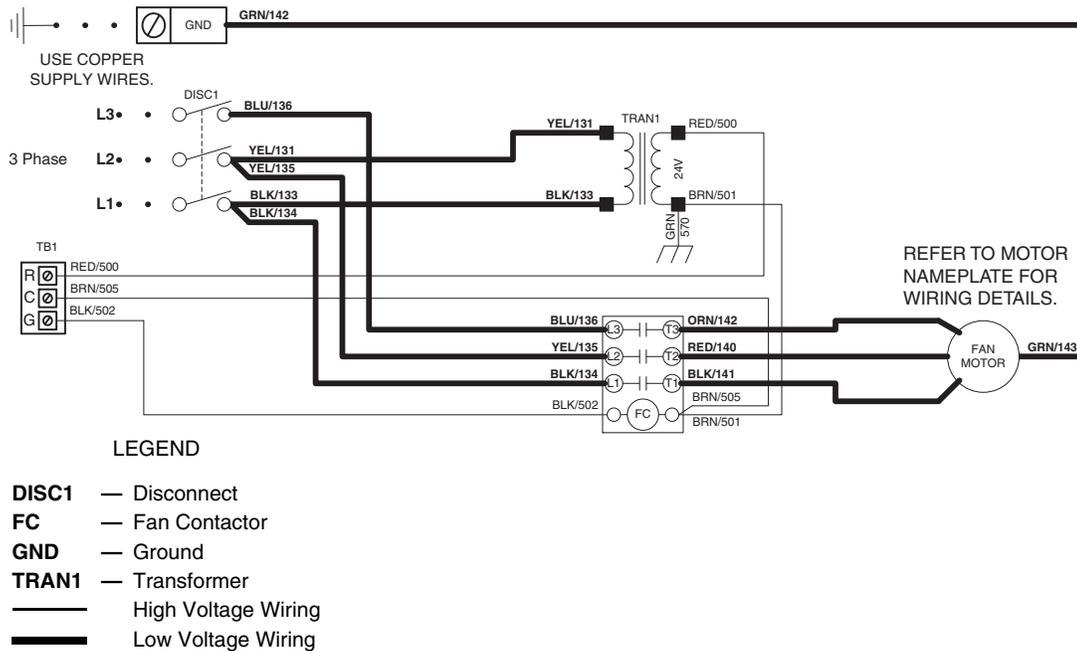
**Fig. 95 — Typical Wiring Diagram, Three-Phase Contactor Control**
