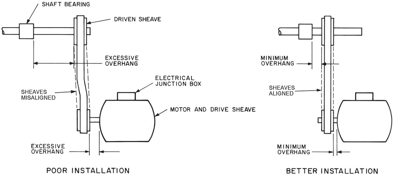
**Fig. 63 — Determining Sheave-Shaft Overhang**
