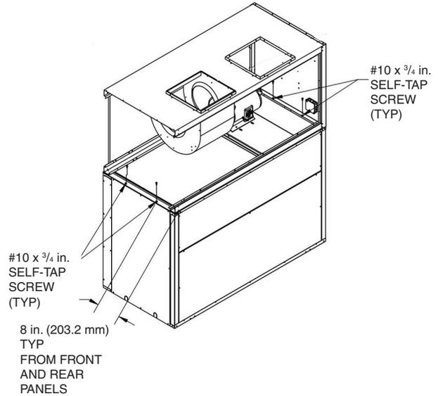
**Fig. 27 — Connect Sections with Screws**
