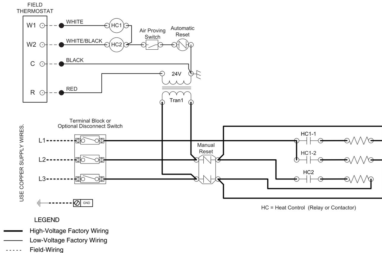
**Fig. 83 — Electric Heat Wiring Schematic, Dual Point Power (Delta Wiring), 240V 3-Phase 11 to 17 kW and 480V 3-Phase 21 kW**
