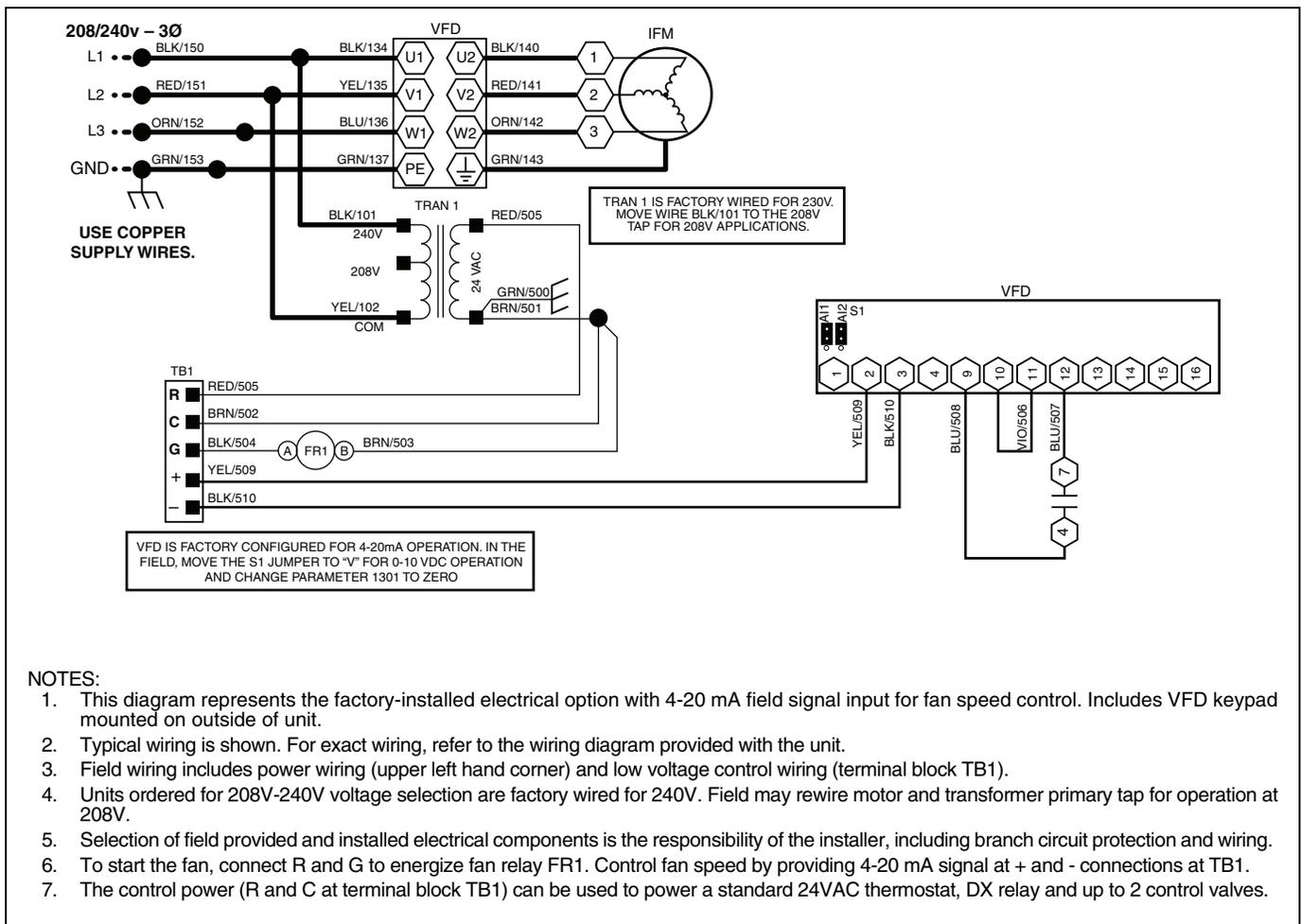
**Fig. 87 — Control Option “A,” 4-20 mA Fan Speed Control Typical Wiring Diagram**
