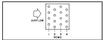
Above is a 4-row coil with a 4-tube face. Note that tubes are staggered in adjacent rows.
