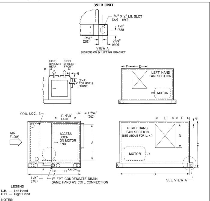
Hand is determined by the location of the fan drive and/or coil connection when viewed while facing the direction toward which air is flowing.
