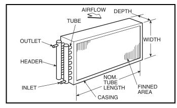
**Header** — The header is a pipe of large diameter to which several tubes are connected. It serves as a distributor of the heating or cooling medium to the tubes. Headers are typically of non-ferrous metal or steel.
