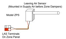
NOTE: If the ZPS is not used, the NO SENSOR jumper located just above the LAT terminals must be on the pins.
