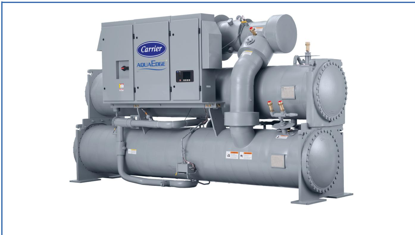
**Low harmonic distortion option (with LF-2 VFD)** — The AquaEdge 23XRV chiller will generate less than 5% total harmonic distortion at the input to the VFD (variable frequency drive) without the use of any external filters or line reactors. This assures the VFD alone cannot exceed IEEE-519 standard for distortion at the point of common coupling. Ultra-low harmonics can eliminate need for complicated harmonic system studies.
