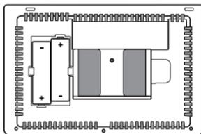
**For battery power**, insert the 2 supplied "AA" type alkaline batteries into the battery compartment located in the rear housing of the thermostat. Make sure to position the Positive (+) and Negative (-) sides of the batteries correctly with the +/- symbols in the battery compartment.
