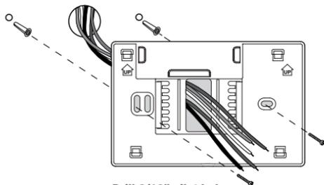
Drill 3/16" pilot holes in your desired location. Use supplied anchors for drywall or plaster.
