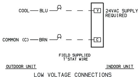
Fig. 5 – 24AHA4 Typical Control Circuit Connections
