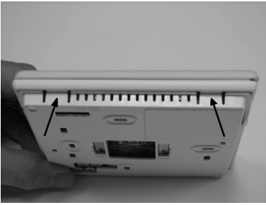
Fig. 4 - Press Tabs to Remove Backplate
