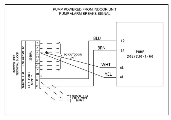
Fig. 12 - (208/230-1-60) WIRING SCHEMATIC
