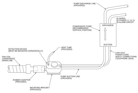
Fig. 7 – Accessory Condensate Pump Connections
