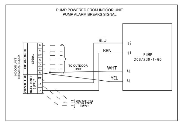
Fig. 13 - (208/230-1-60) WIRING SCHEMATIC
