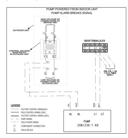
Fig. 22 - 208/230-1-60 Pump in a 208-230-1-60 40MK\*B high wall AC unit - WIRING SCHEMATIC
