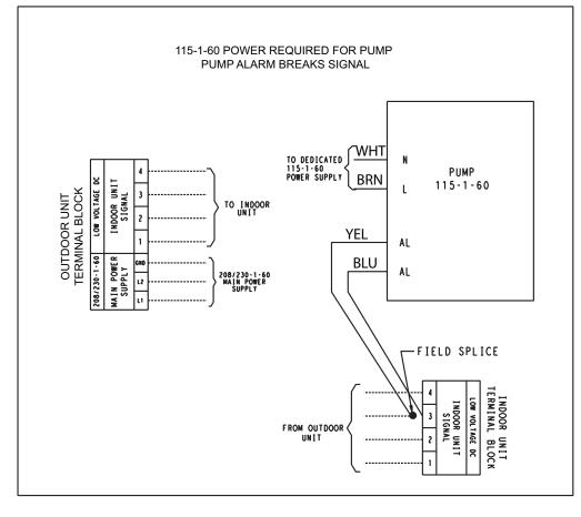
Fig. 9 - Installing a 115-1-60 Pump in a 208/230-1-60 unit-WIRING SCHEMATIC
