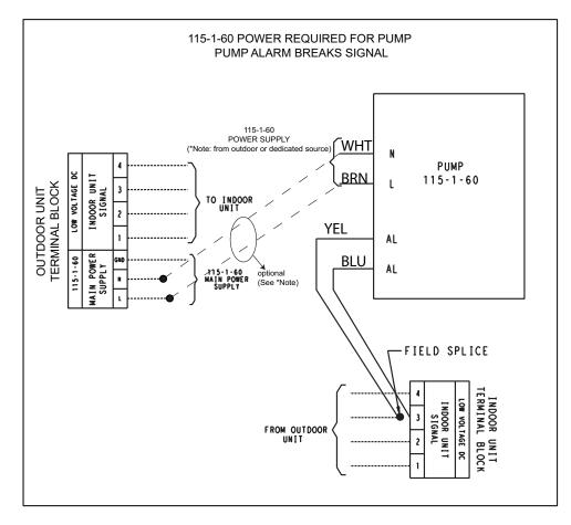
Fig. 8 – (115-1-60) WIRING SCHEMATIC
