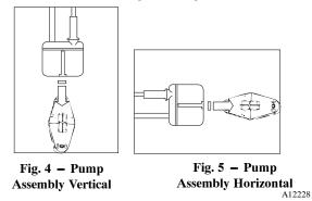
If the pump is not mounted in the vertical position, make sure that plug on the pump is above the refrigerant tubing. This is required to avoid water leaking onto the pump causing a short circuit. **The pump cannot be splashed nor located in a damp environment.**
