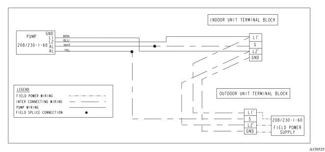
Fig. 29 - Sizes 09&12 (208-230-1-60) 40GRQ / 619FB High Wall HP Unit - WIRING SCHEMATIC
