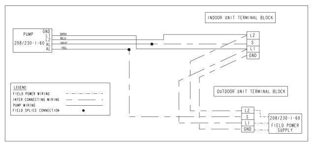
Fig. 18 - (208/230-1-60) WIRING SCHEMATIC
