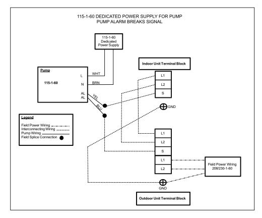
Fig. 14 – Installing a 115-1-60 Pump in a 208/230-1-60 unit-WIRING SCHEMATIC
