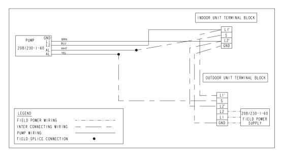
Fig. 30 - Size 18 (208-230-1-60) 40GRQ/619FB High Wall HP Unit - WIRING SCHEMATIC
