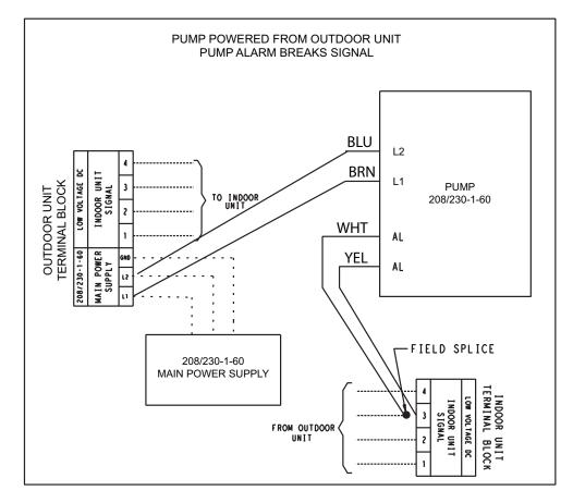
Fig. 10 - (208/230-1-60) WIRING SCHEMATIC
