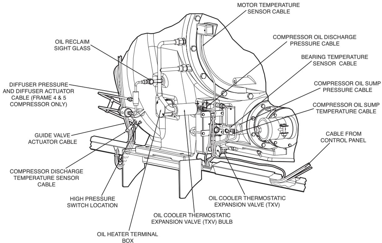
**Fig. 12 — 19XR,XRV Compressor Controls and Sensor Locations**
