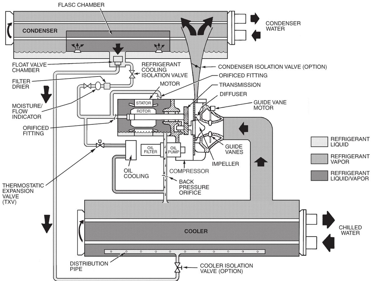
Fig. 4 — Refrigeration Cycle — 19XR,XRV Single-Stage Compressor
