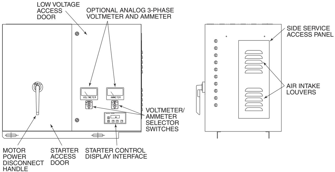
**Fig. 10 — Typical Starter External View (Solid-State Starter Shown)**
