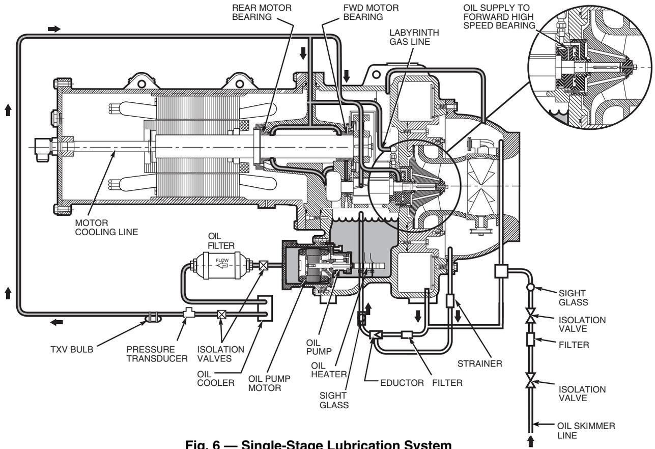
**Fig. 6 — Single-Stage Lubrication System**
