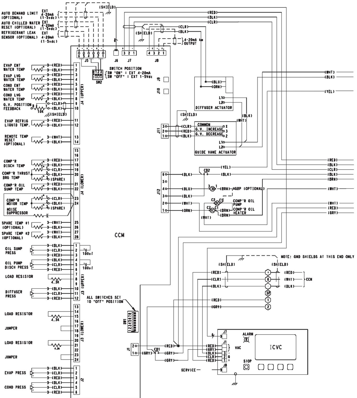
Fig. 63 — PIC II Control Panel Wiring Schematic (Frame 4 and 5 Compressors with Split Ring Diffuser)
