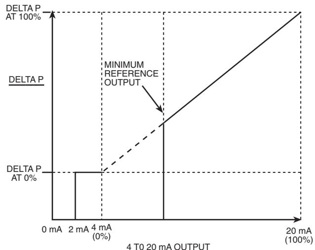
Fig. 28 — Head Pressure Reference Output (Minimum Set Above 4 mA)
