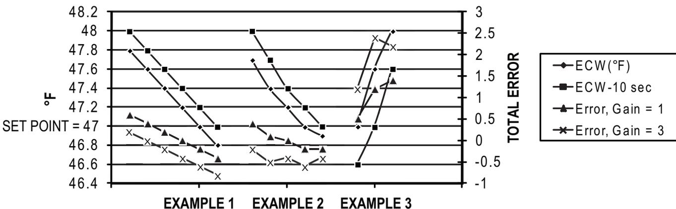
**Fig. 24 — Transient Example of ECW Gain**
