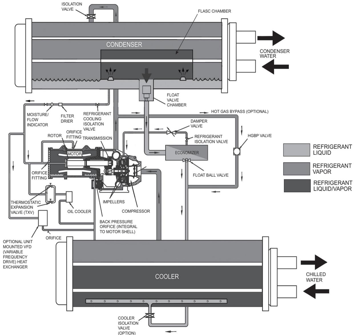
**Fig. 5 — Refrigeration Cycle — 19XR, XRV Two-Stage Compressor**
