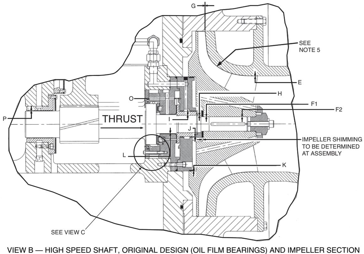
**Fig. 58 — Compressor Fits and Clearances — Single-Stage Compressors (cont)**
