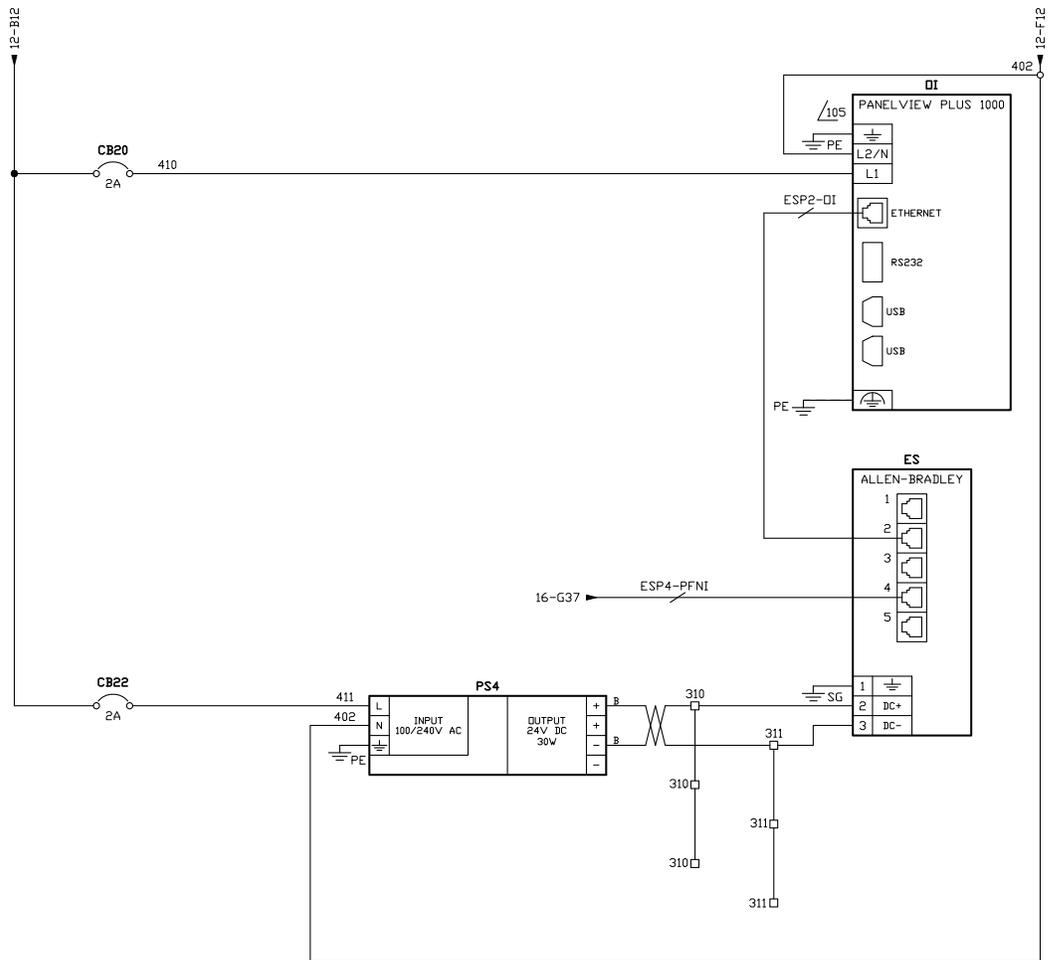
Fig. 71 — Typical Medium-Voltage Variable Frequency Drive (VFD) Wiring Schematic (cont)
