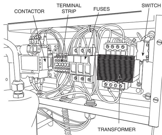
**Fig. 53 — Pumpout Control Box (Interior)**
