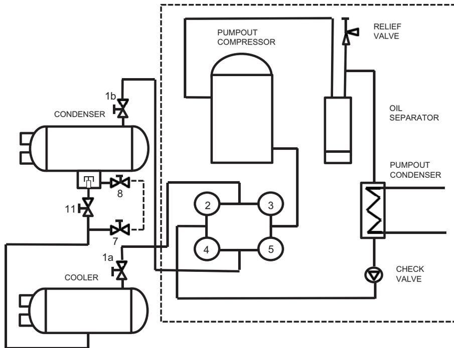
**Fig. 44 — Typical Optional Pumpout System Piping Schematic without Storage Tank**
