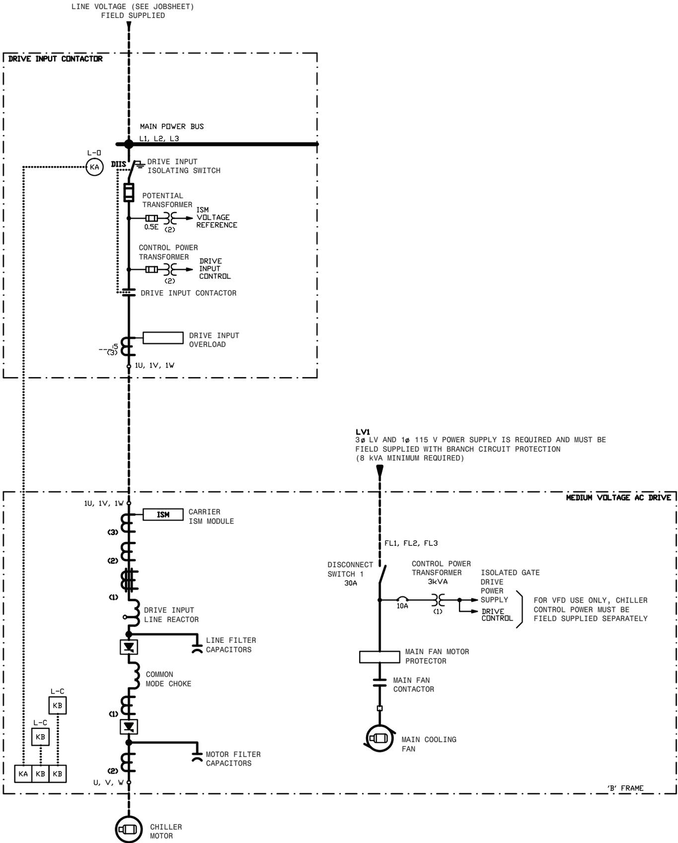
Fig. 71 — Typical Medium-Voltage Variable Frequency Drive (VFD) Wiring Schematic
