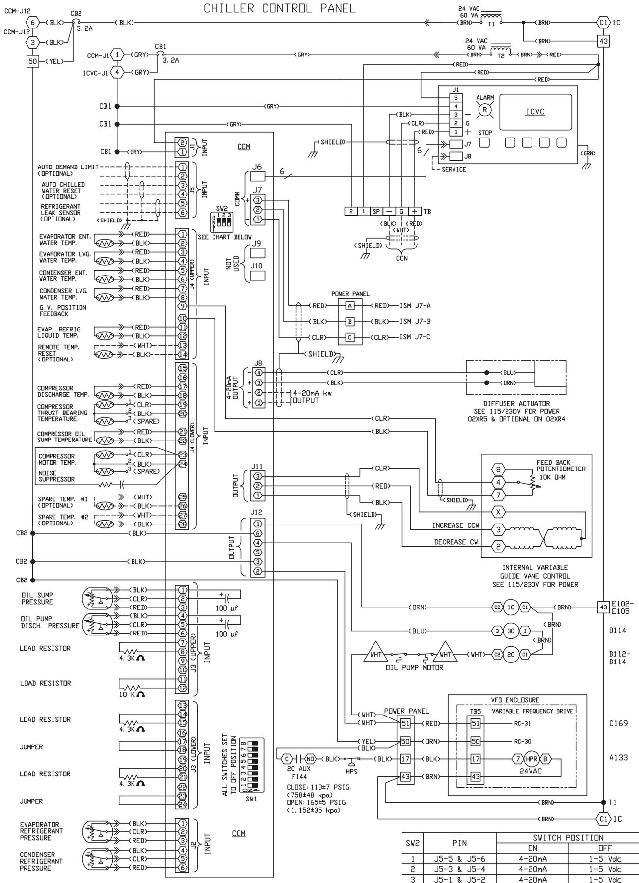
Fig. 69 — Typical Low-Voltage Variable Frequency Drive (VFD) Wiring Schematic (575 v) (cont)
