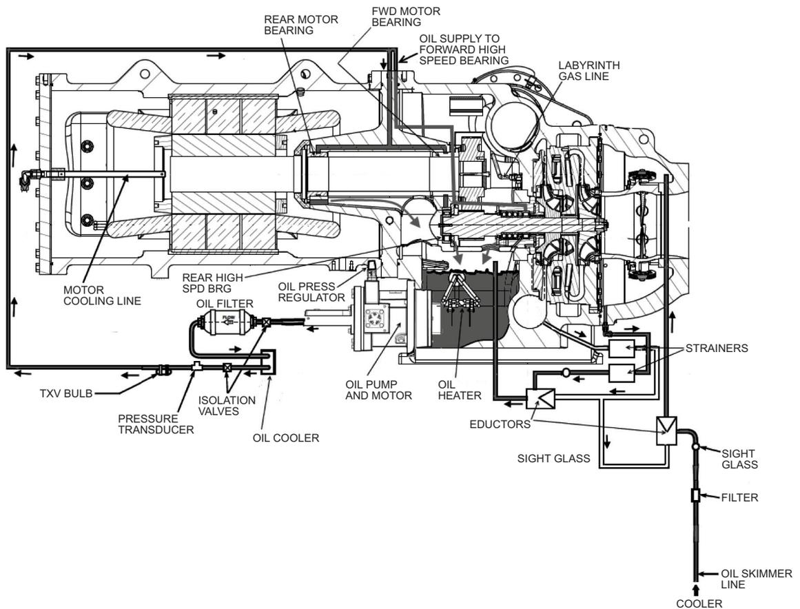
**Fig. 7 — Two-Stage Lubrication System**
