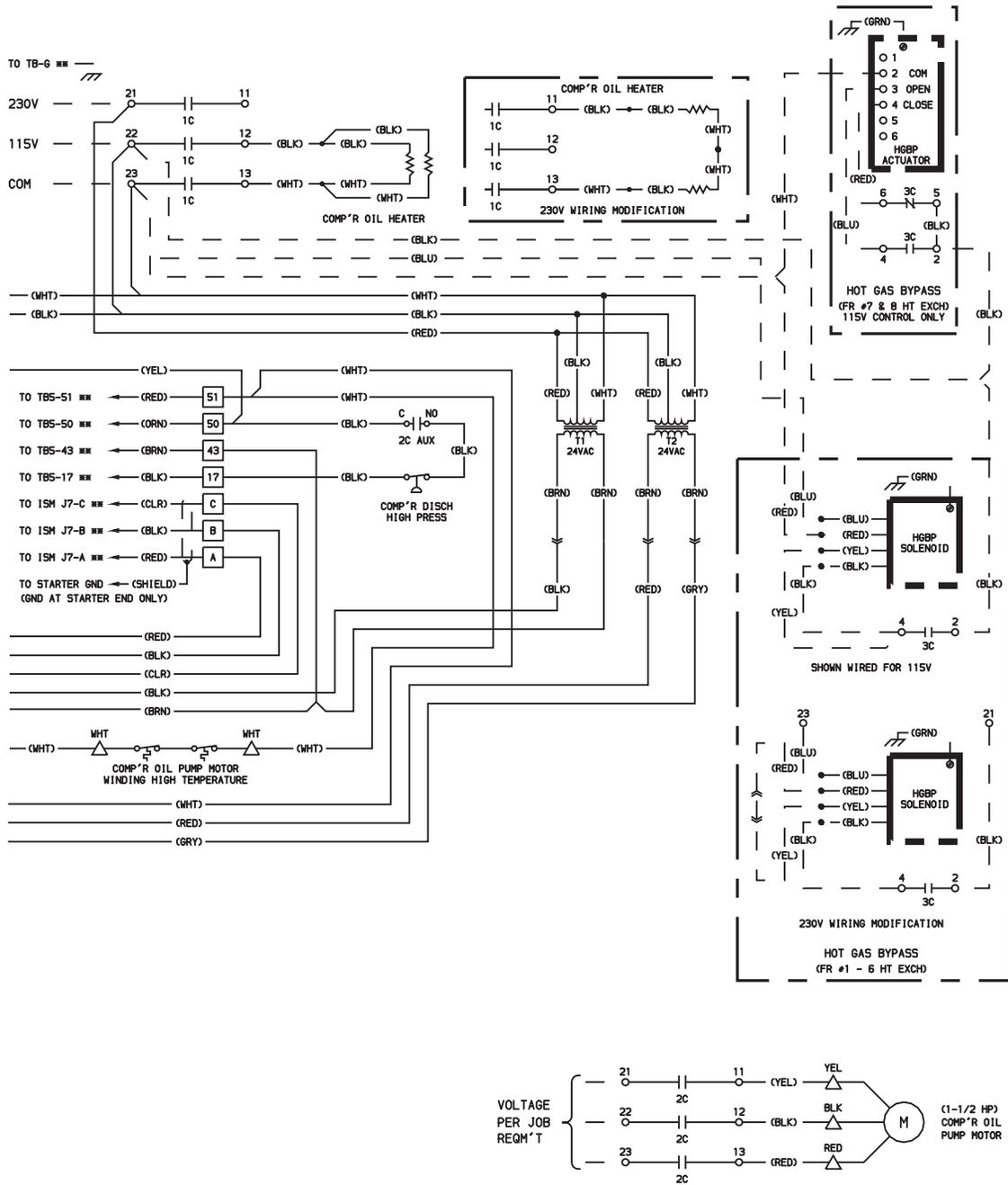
Fig. 62 — PIC II Control Panel Wiring Schematic (Frame 2, 3, 4 and E Compressors without Split Ring Diffuser) (cont)
