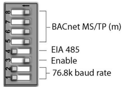
**Fig. C — DIP Switches**
