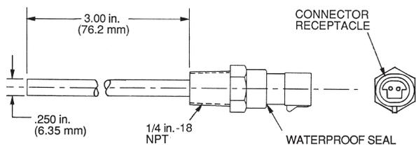
**Fig. 15 — Control Sensors (Temperature)**
