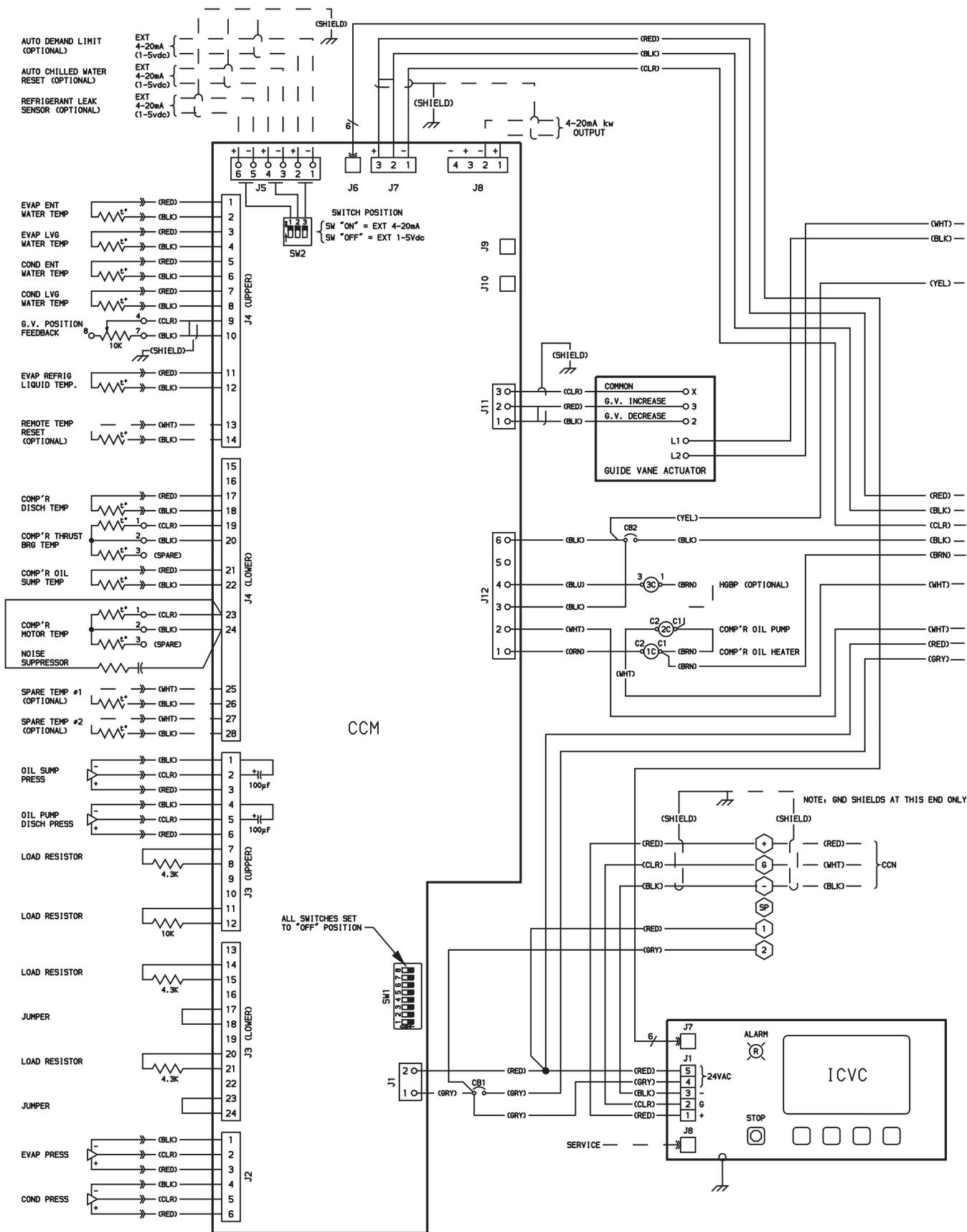
Fig. 62 — PIC II Control Panel Wiring Schematic (Frame 2, 3, 4 and E Compressors without Split Ring Diffuser)
