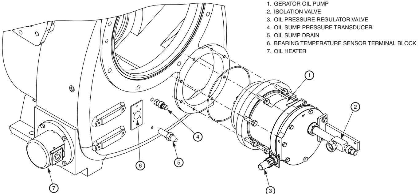
**Fig. 8 — Gerotor Oil Pump**
