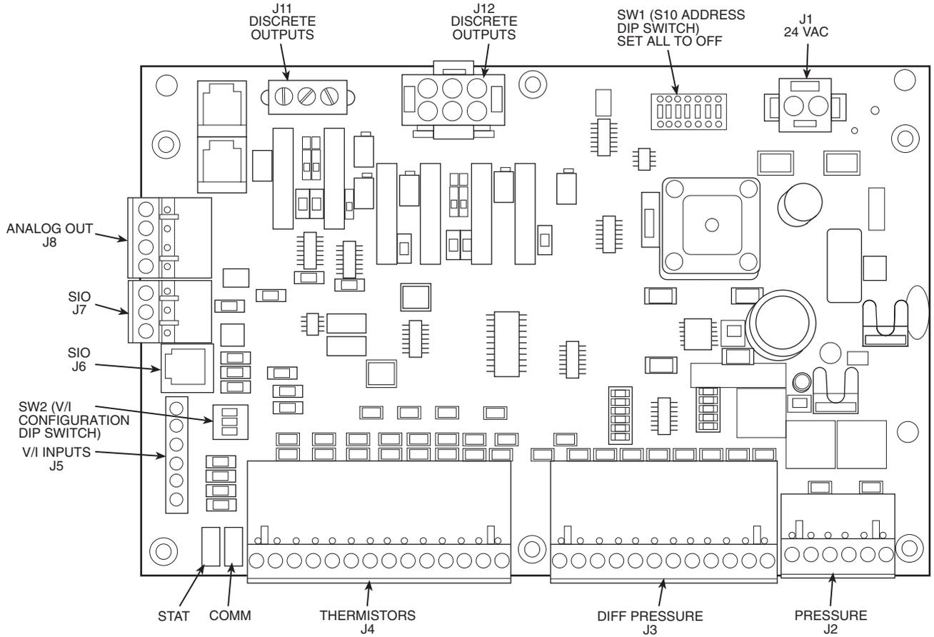
**Fig. 55 — Chiller Control Module (CCM)**
