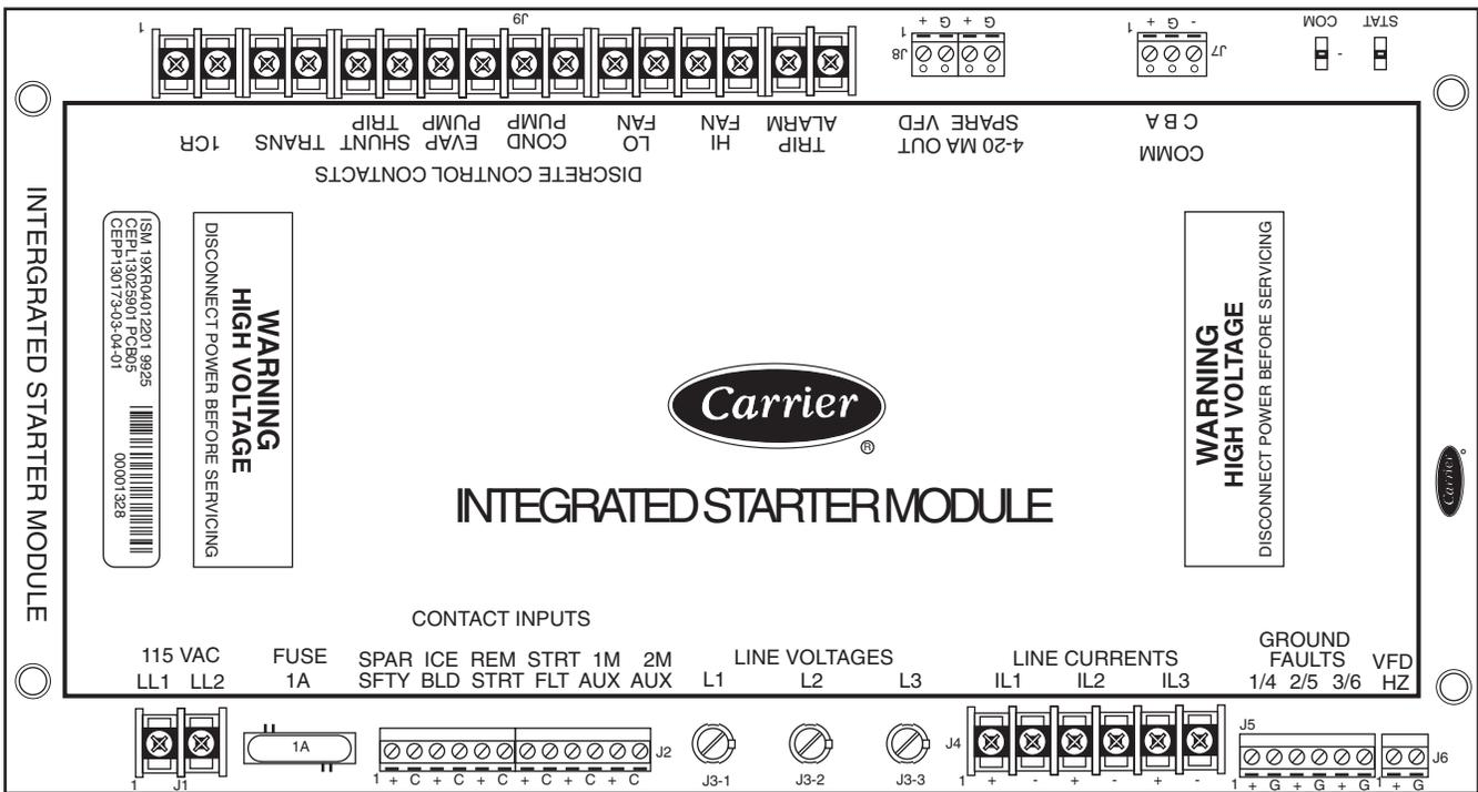
**Fig. 56 — Integrated Starter Module (ISM)**
