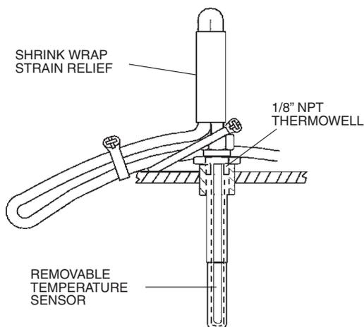
**Fig. 16 — Temperature Sensor Used with Thermal Well**
