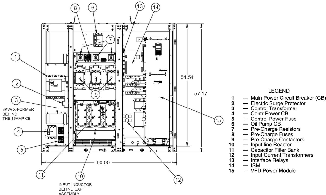
**Fig. 11 — PIC II Unit-Mounted 575-v Variable Frequency Drive (VFD) Internal View**
