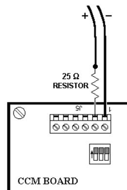
**Fig. 26 — Auto Demand Limit Wiring (1 to 5 vdc)**
