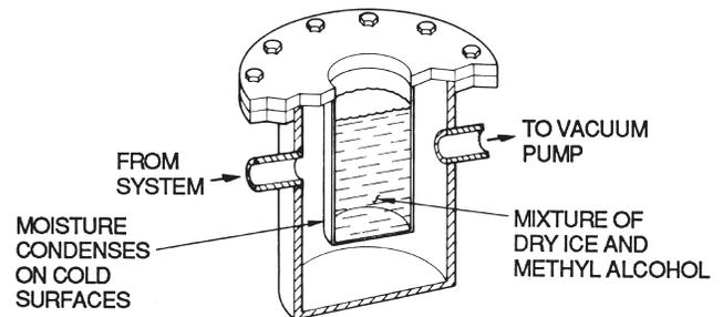
**Fig. 34 — Dehydration Cold Trap**
