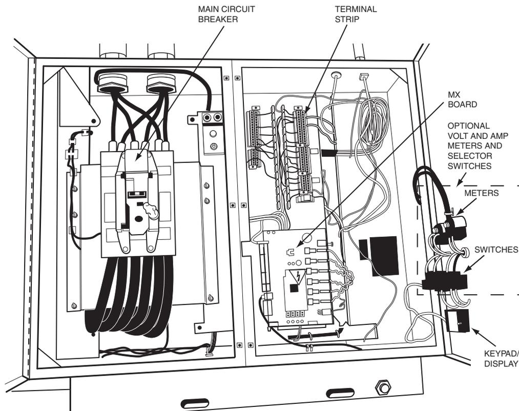
**Fig. 9 — Benshaw Solid-State Starter, Internal View**
