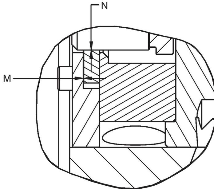
VIEW C — HIGH SPEED SHAFT RING SEAL
