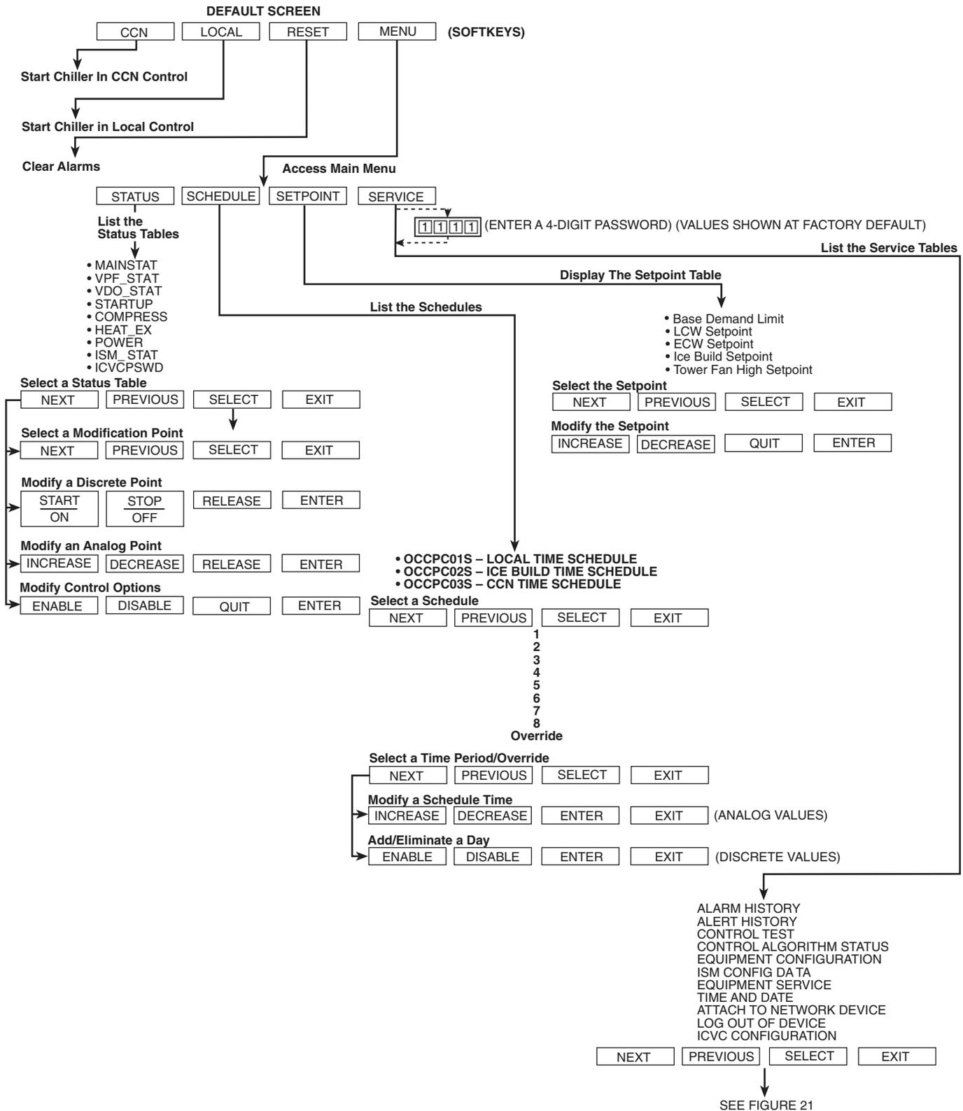
**Fig. 20 — PIC II19XR,XRV Chiller Display Menu Structure for ICVC Software Version 14**
