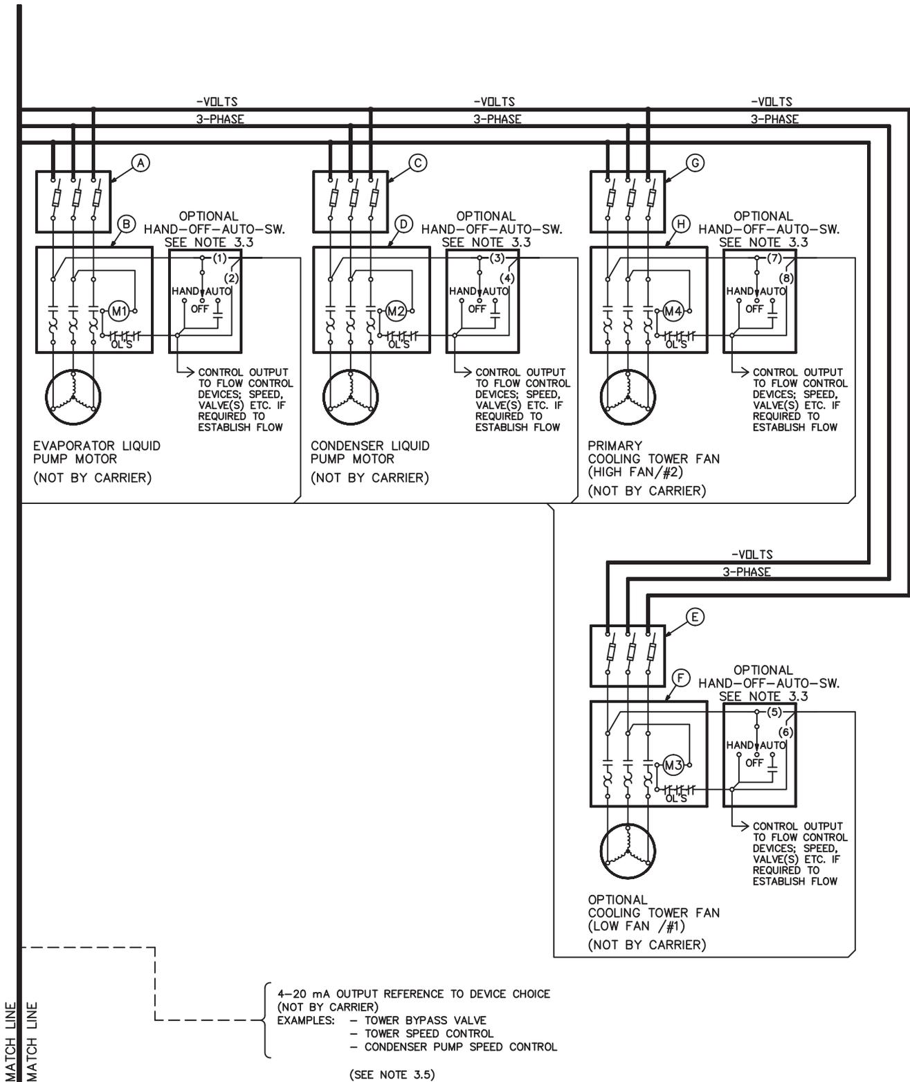
**Fig. 70 — 19XR Typical Wiring with Unit-Mounted Variable Frequency Drive with ISM (Integrated Start Module) (cont)**
