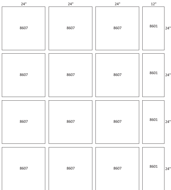
UNIT SIZE 51T (12) 24" X 24" FILTERS (4) 12" X 24" FILTERS
